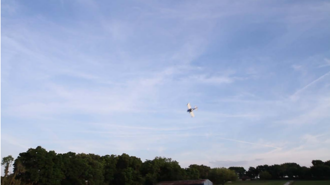
Image 1 – The airplane is low, about 20 degrees nose down and 90 degrees left wing down.
