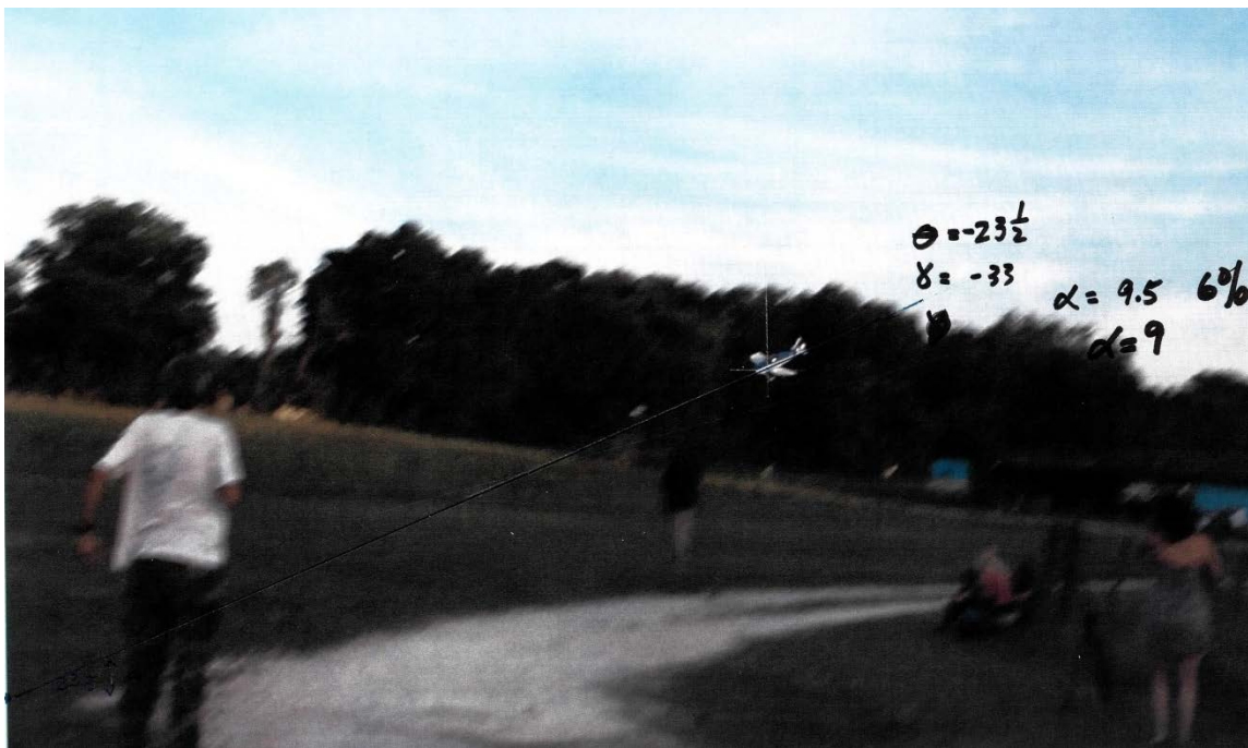
Image 4 - The measured flight path is -33 degrees. The measured pitch attitude is -23.5 degrees. The difference is a perceived angle of attack of 9.5 degrees. The airplane is about 20 degrees from perpendicular to the viewing angle. The corrected angle of attack is 9 degrees.
