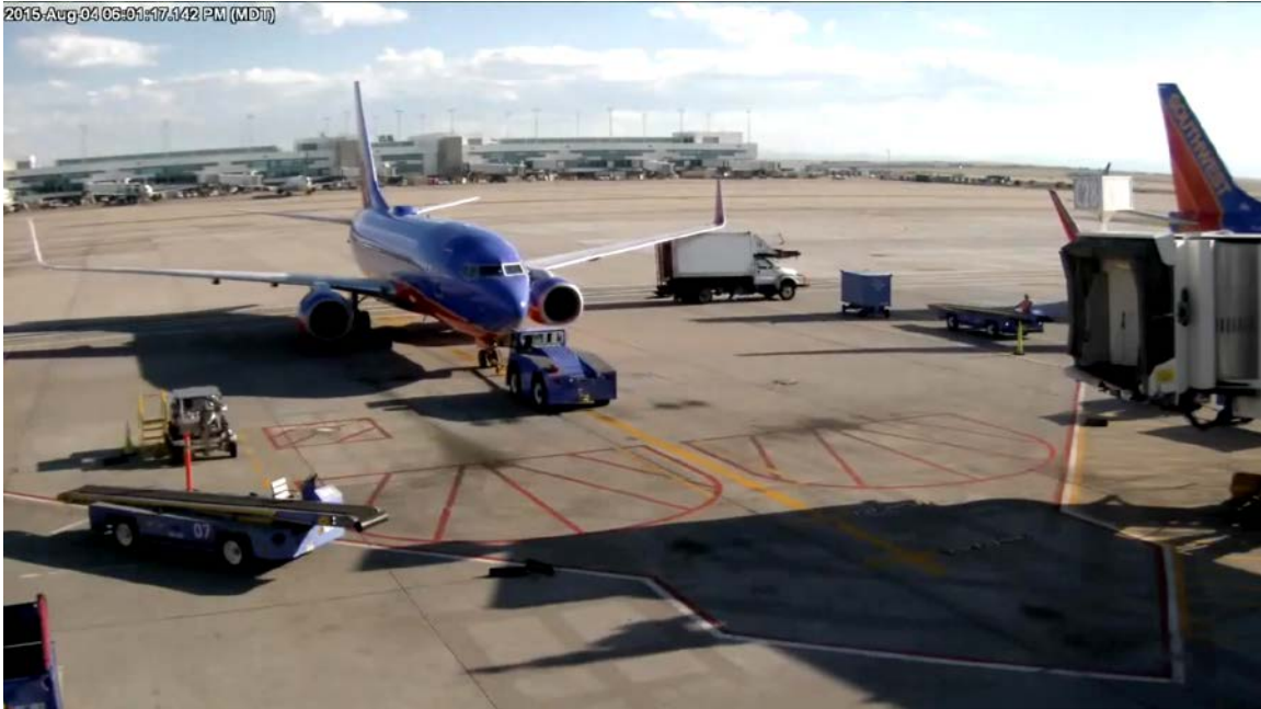
Photograph 4 - Collision between the left wing and the provisioning truck
