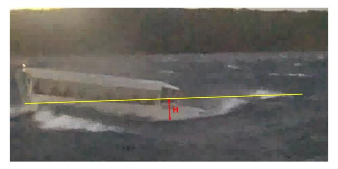
Figure 10. Wave Height Estimation
