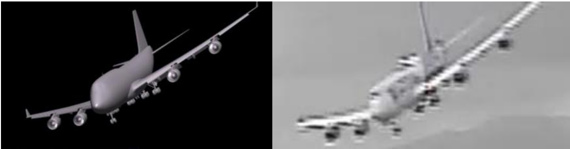
Figure 14. A textured model rendered of the aircraft next to the enlarged raw image file in frame 08 from the accident video.
