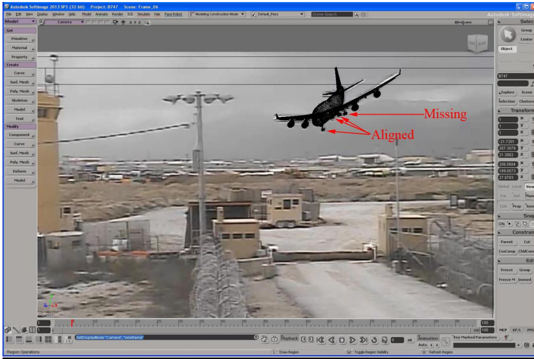
Figure 16. A wireframe model aligned to frame 10 in Autodesk Softimage.
