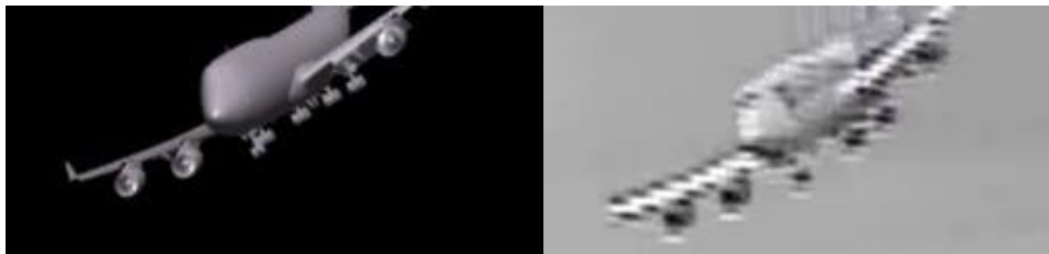
Figure 11. A textured model rendered of the aircraft next to the enlarged raw image file in frame 06 from the accident video.
