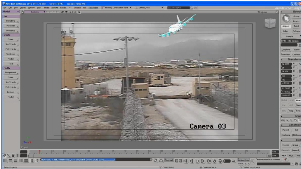
Figure 10. A wireframe model aligned to frame 06 in Autodesk Softimage.
