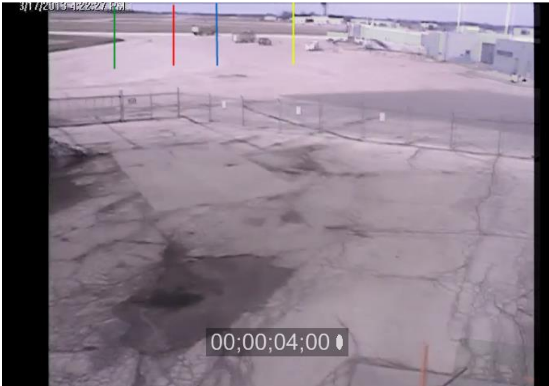
Image 4.19: Vertical lines drawn from each of the known calibration positions are used to indicate when the accident aircraft crossed each segment on the runway's centerline in reference to the security camera's perspective. In this image both the calibration recording and the accident recording are overlaid on each other with an opacity value set to 50%. A time code was added in a 30 frame per second SMPTE 8 timecode format.
