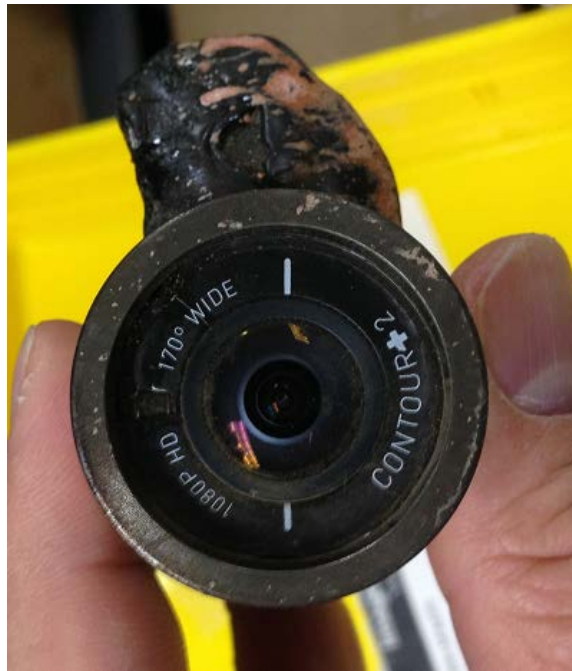
Figure 4. Contour+2 after damaged lens removed.
