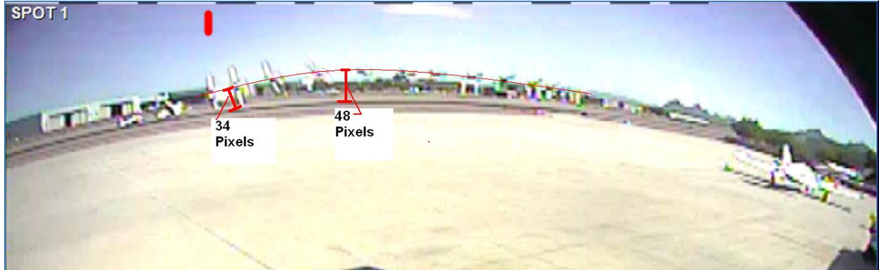
Figure 1. FBO security video time-lapse representation with annotations of curved path and vertical measures.
