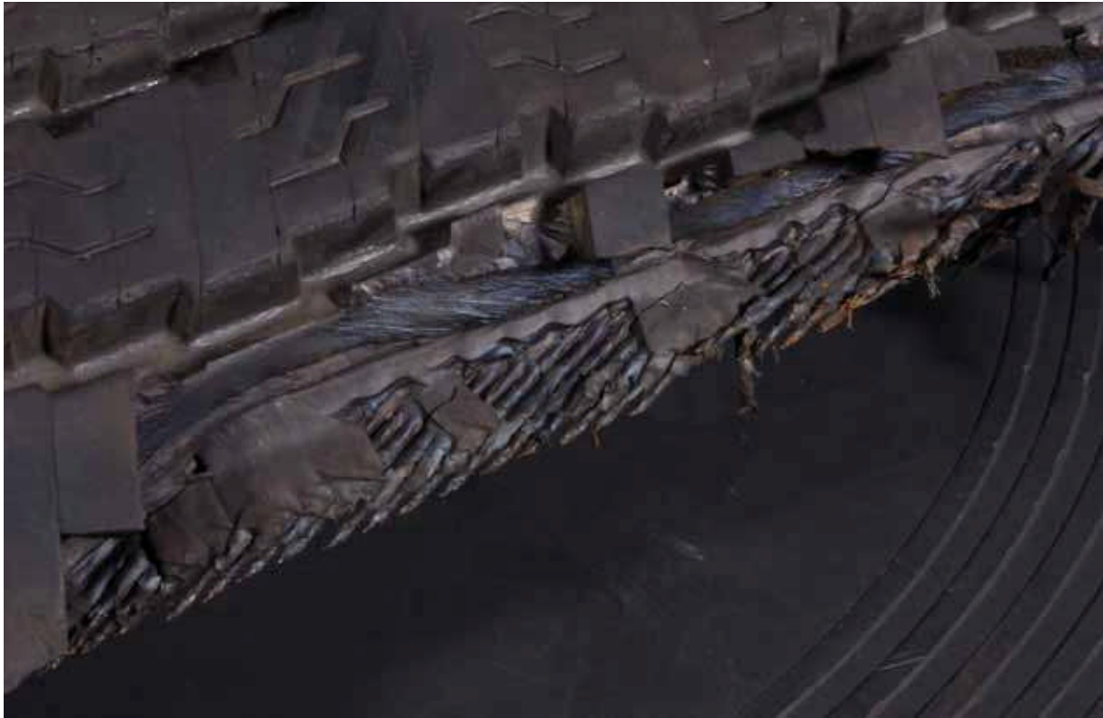
Figure 8: Torn Appearance of 3 rd Belt Edge, Serial Side, about 7:00 (08AA330-B142.jpg)
