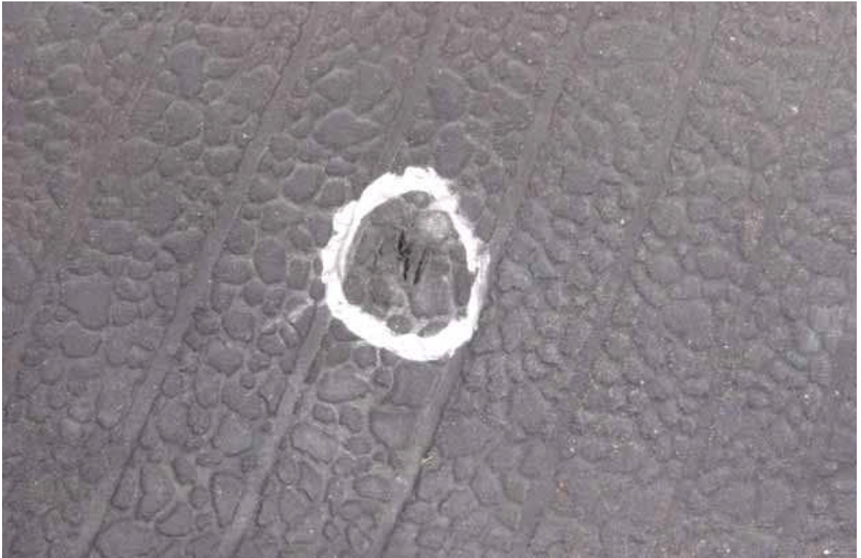
Figure 14: Penetration Tears to Innerliner, about 4:00, Serial Side Shoulder (08AA330-B257.jpg)
