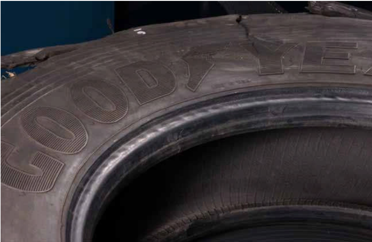
Figure 11: Rim Flange Compression Grooving, Serial Side (08AA330-B134.jpg)
