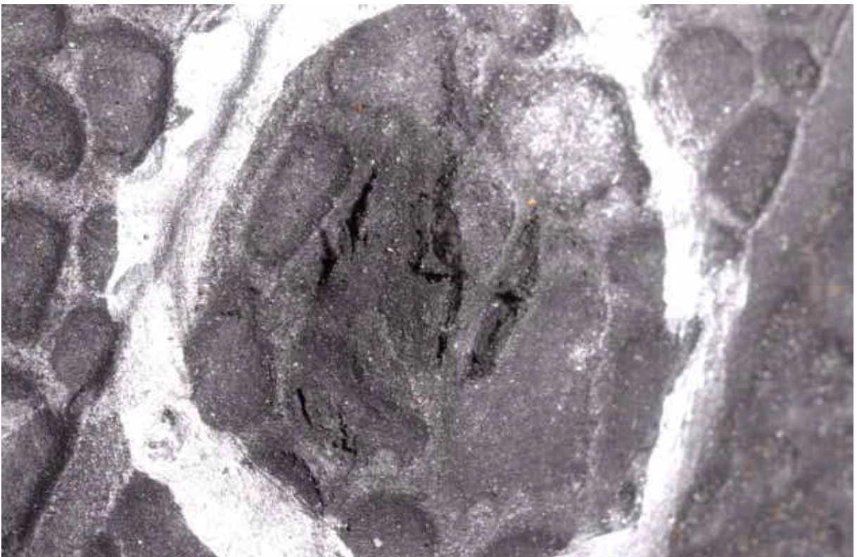
Figure 15: Close View of Penetration Tears to Innerliner (08AA330-B259.jpg)
