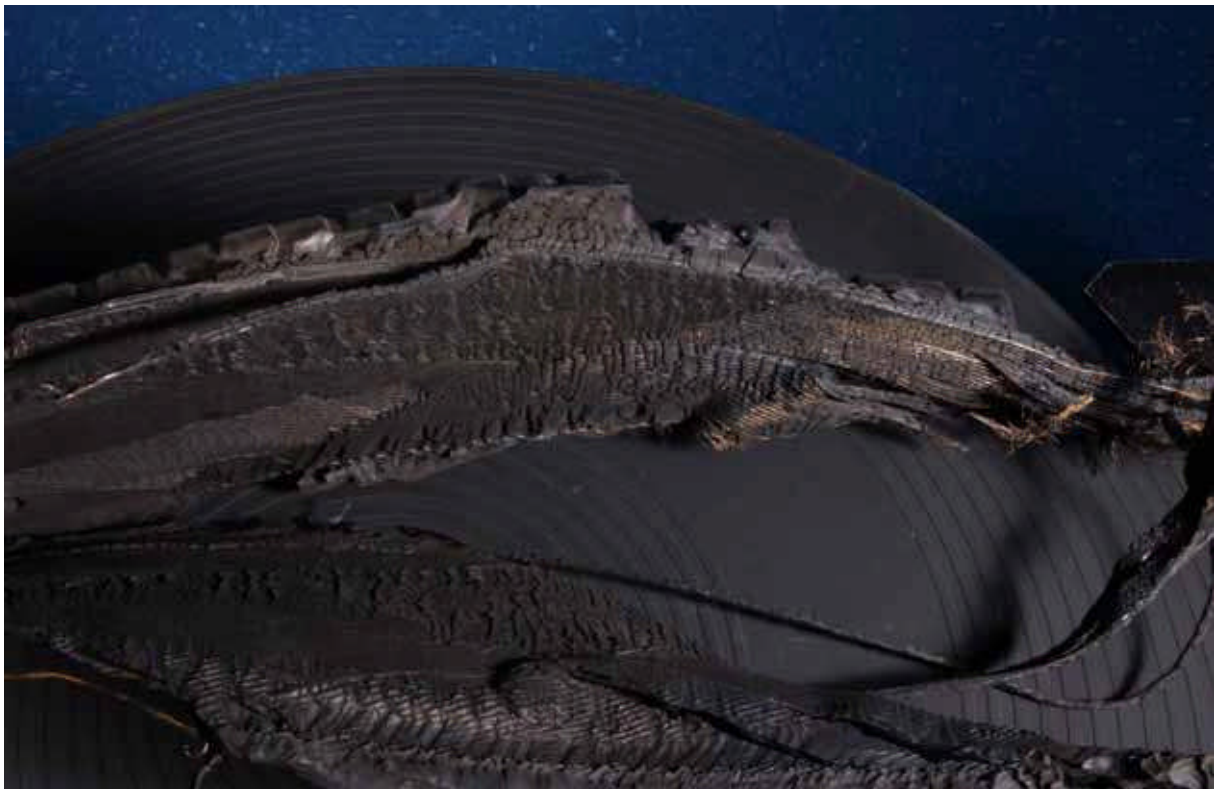
Figure 7: Torn Appearance Between 2 nd and 3 rd Belts, ~9:00 Clockwise to 11:00 (08AA330-B146.jpg)
