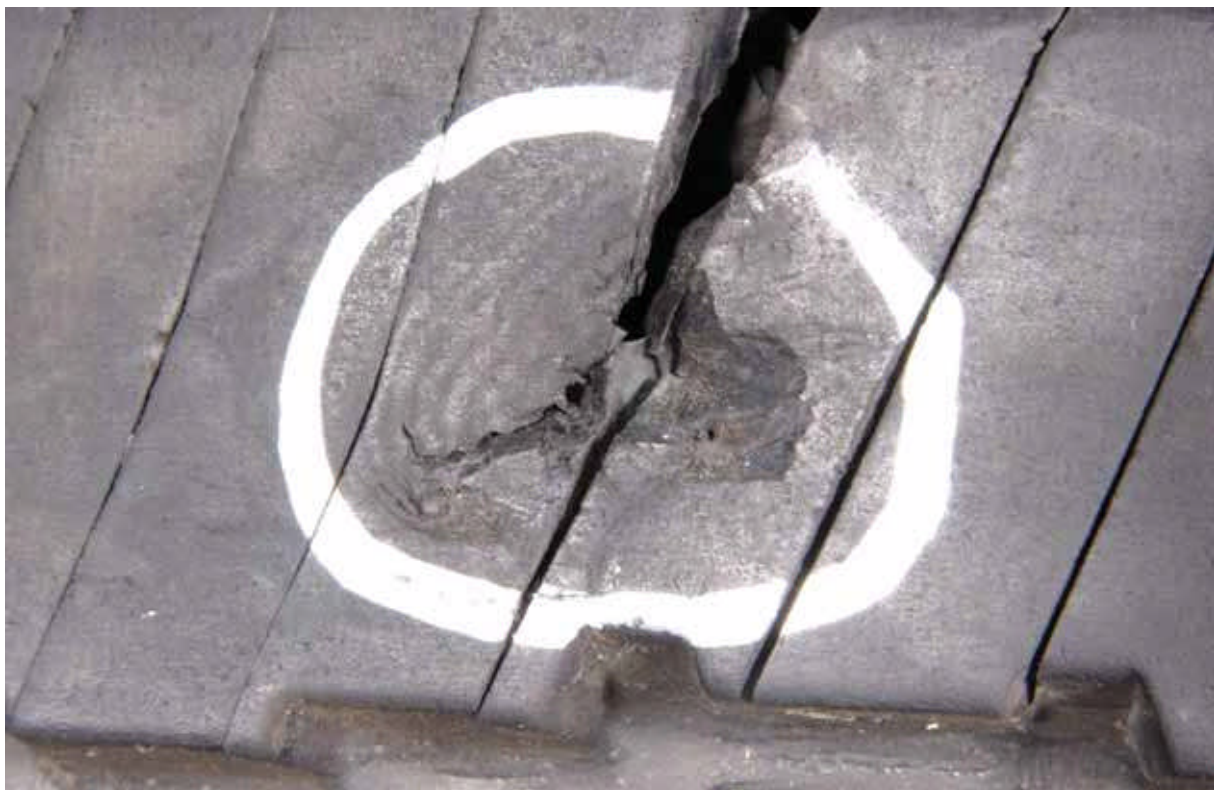
Figure 13: Close View of Puncture Location, about 4:00, Serial Side Shoulder Rib (08AA330-B255.jpg)
