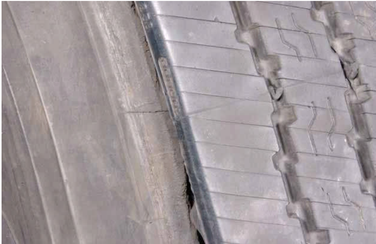
Figure 17: Tread Splice Alignment, Opposite Serial Side Shoulder at 8:30 (08AA330-B208.jpg)
