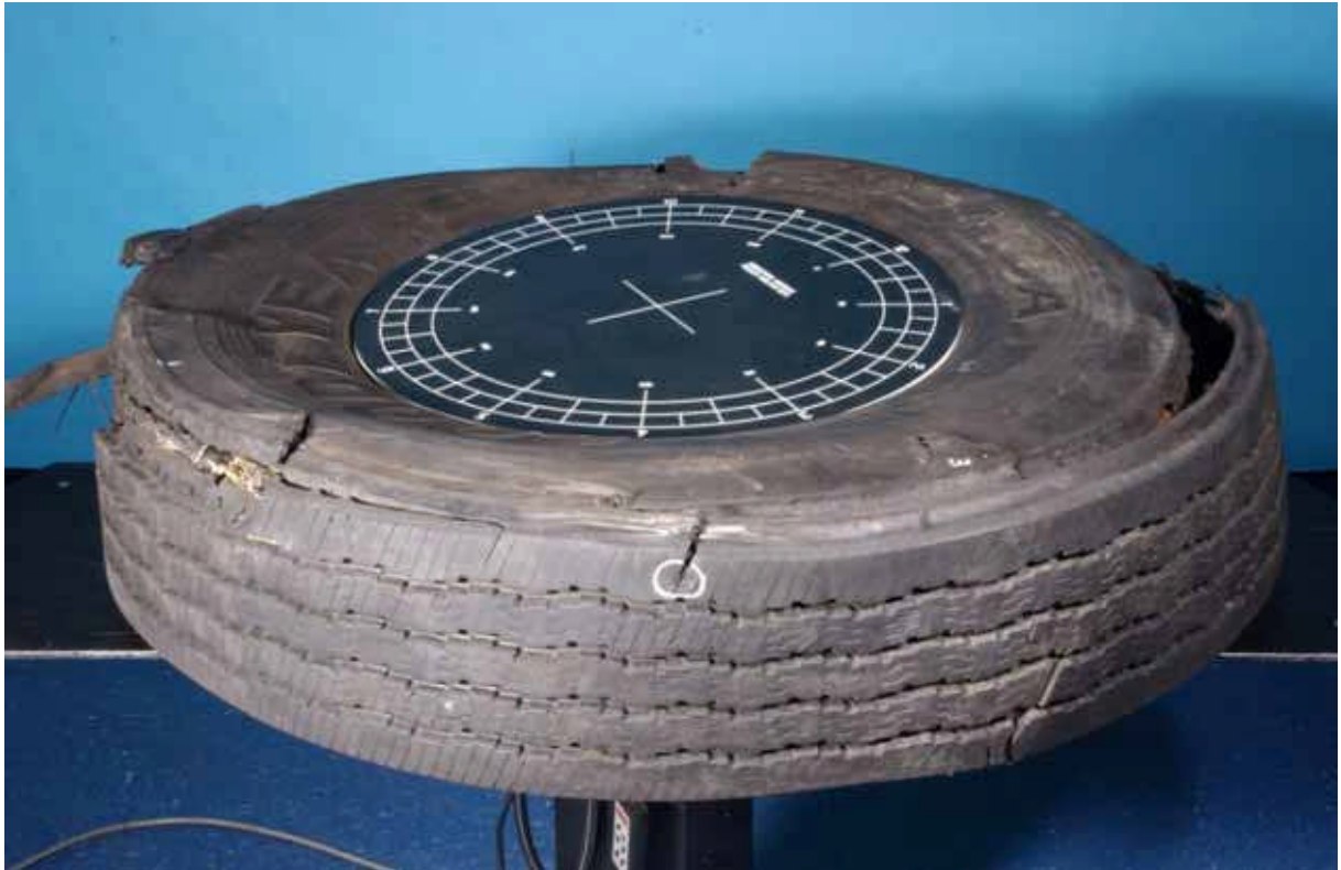
Figure 12: Puncture Location, about 4:00, Serial Side Shoulder Rib (08AA330-B244.jpg)
