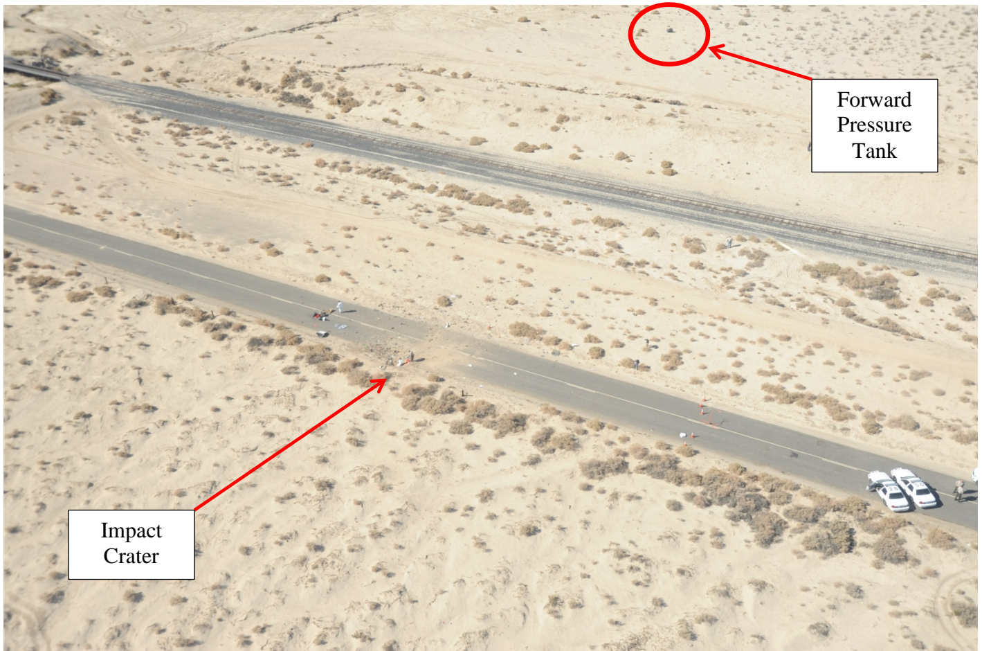
Figure 20 Cockpit section – aerial view of impact crater and forward pressure tank
