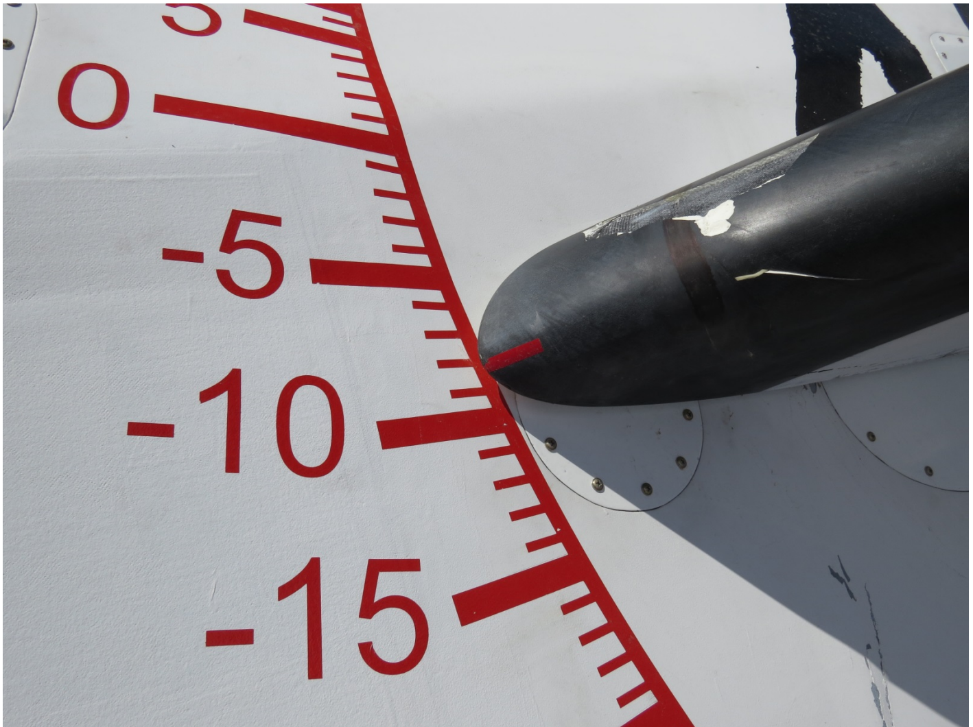
Figure 13 Left boom – horizontal stabilizer reading of -8.5 deg
