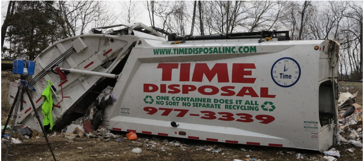
Vehicle Photo 4 – View of the detached refuse hopper of the truck as seen from the right side.
