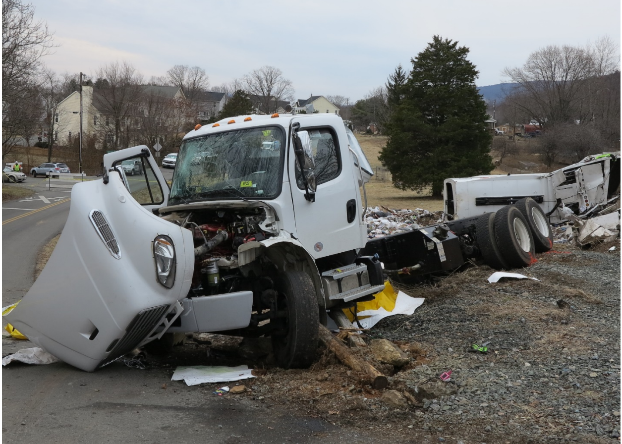
Vehicle Photo #1 – Overall view of the damage to the 2018 Freightliner Refuse Truck facing the left front corner.
