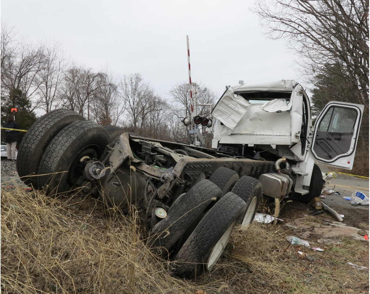
Vehicle Photo #3 – View of the damage to the right side of the refuse truck from the right rear corner.
