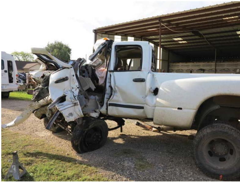
Vehicle Photograph 5 - A Left Side View of the 2007 Dodge Ram 3500 showing the front displacement
