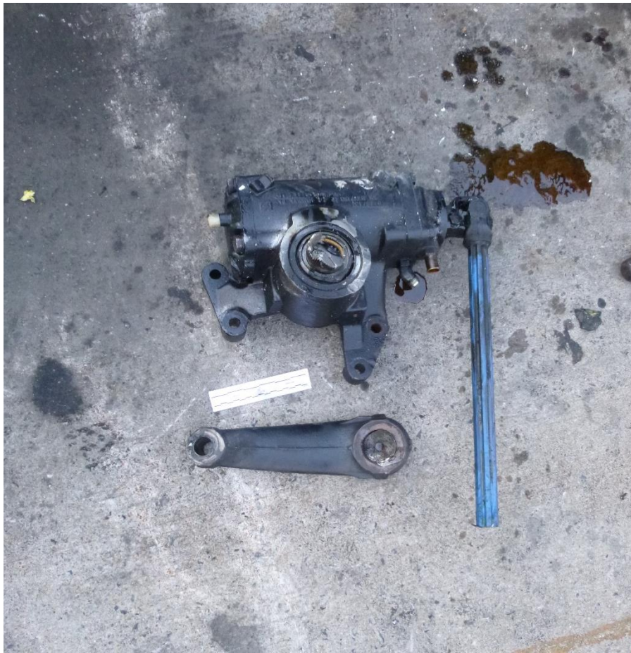
Photo 4 – Steering gearbox from 2015 IC school bus
