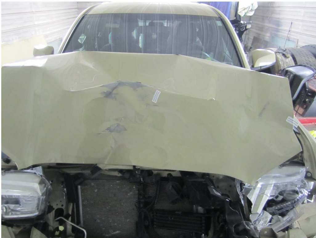
Photo 4. This is a closer view of the damage sustained to the leading edge of the hood.
