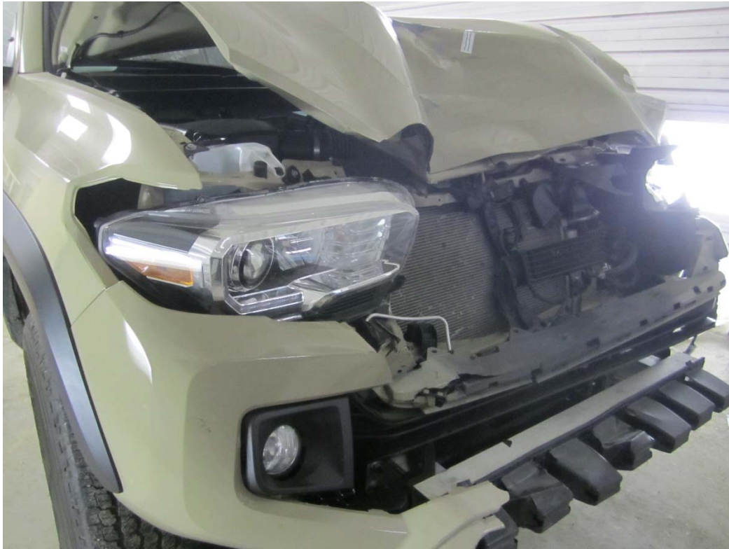
Photo 3. This view is looking at the damage sustained to the right-front of the Toyota pickup.
