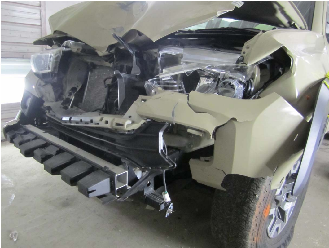
Photo 1. This is a view looking at the damage sustained by the left-front of the Toyota pickup.
