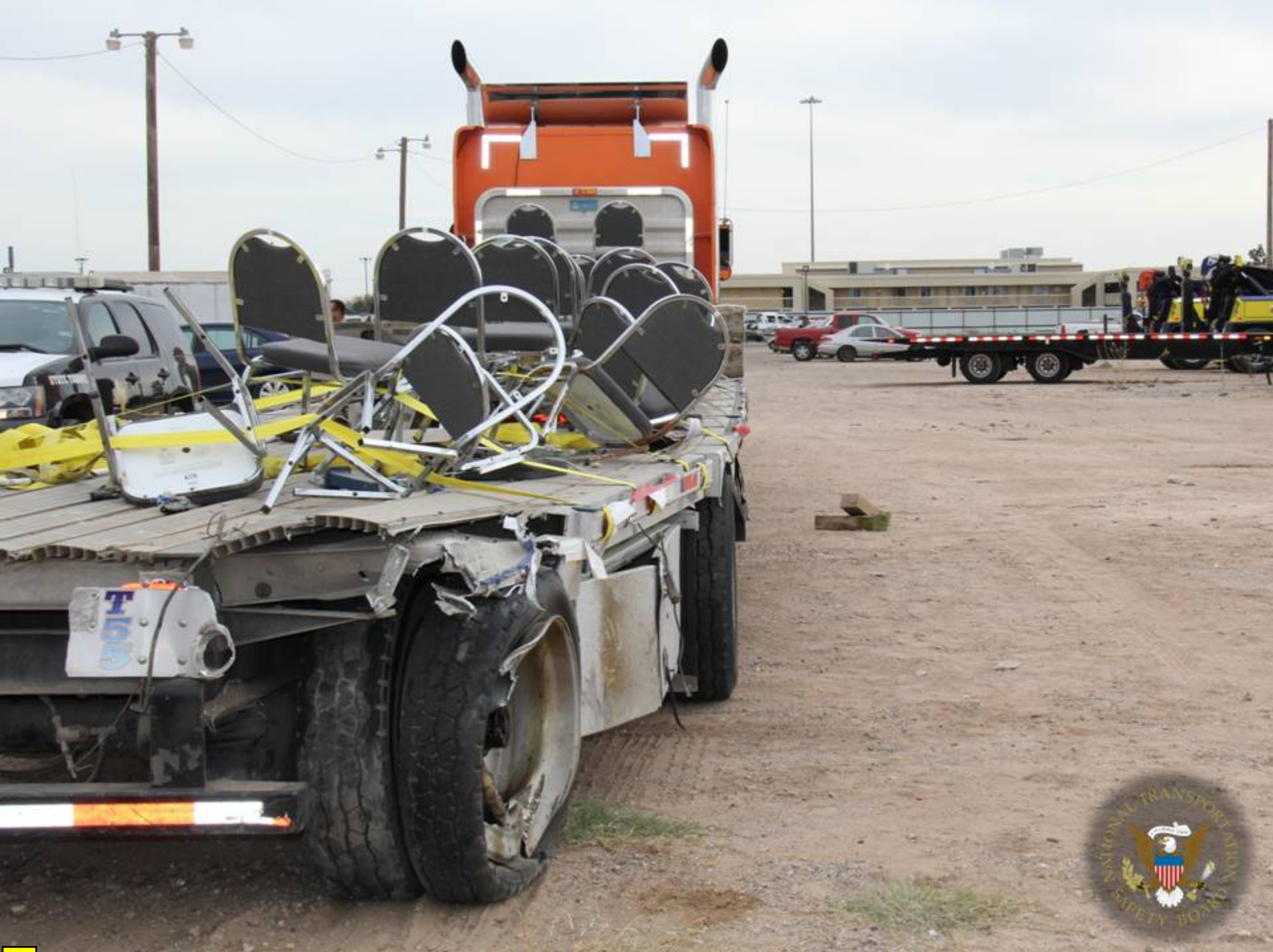
Vehicle Photograph 6 – 2005 Transcraft – Induced Damage to Right Side of Trailer
