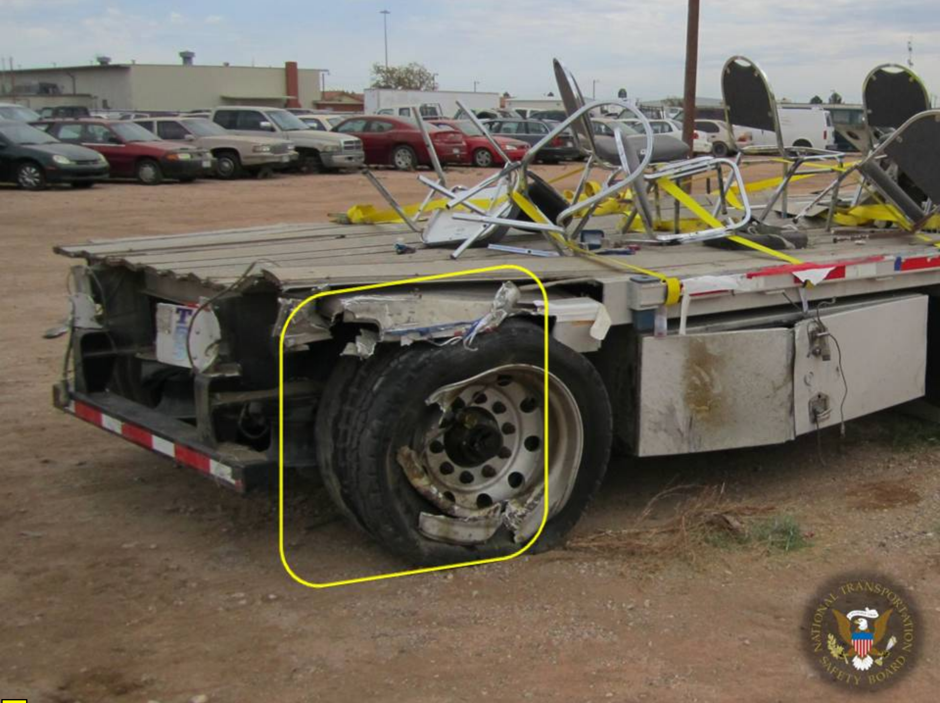
Vehicle Photograph 5 – 2005 Transcraft – Contact Damage to Right Rear Corner
