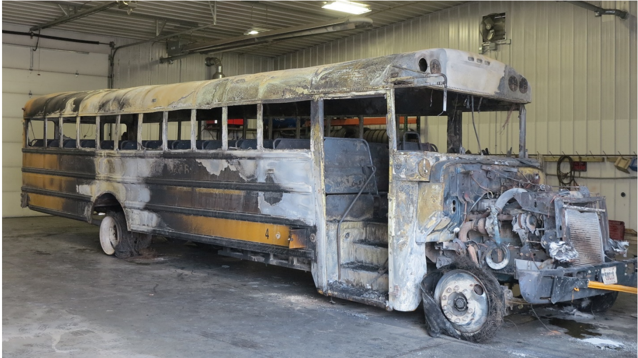
Vehicle Photo #1 – Overall view of the damage to the right side of the 2004 IC School Bus during inspection at Arrow Towing in Council Bluffs, Iowa.
