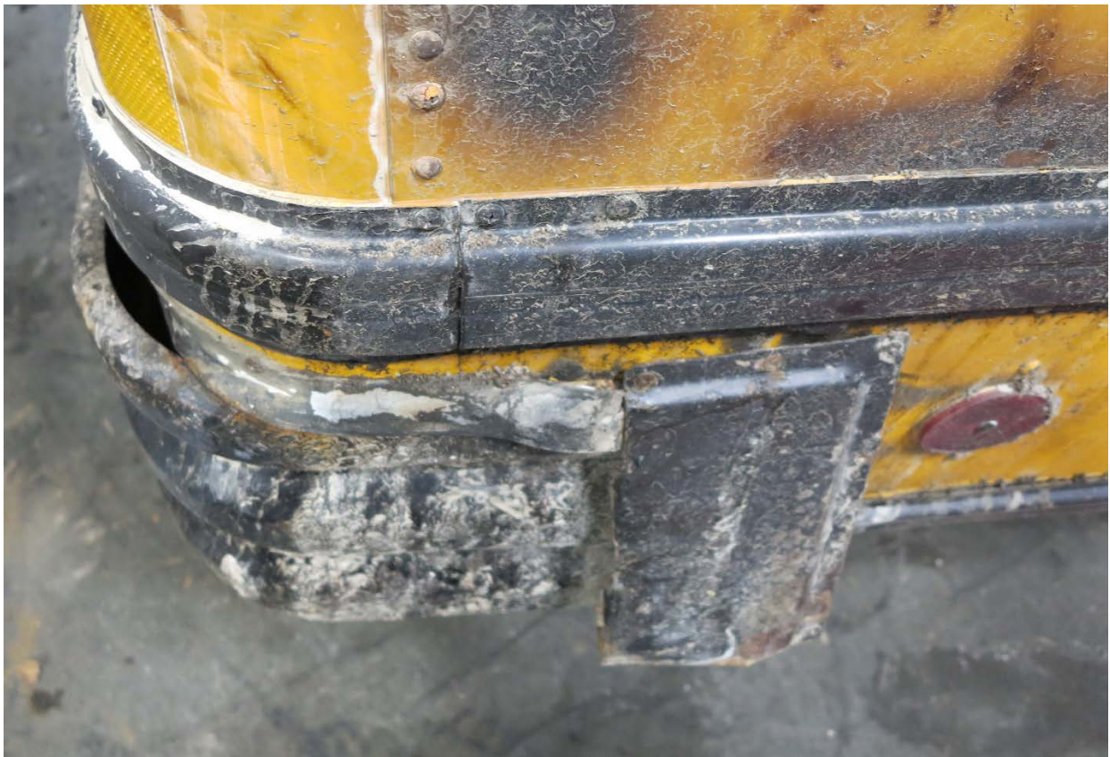
Vehicle Photo #2 – View of the damage to the right rear corner of the school bus.
