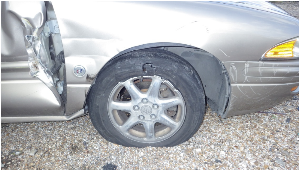
Figure 2. Pattern scratches and tire damage from contact with the HSID bus.
