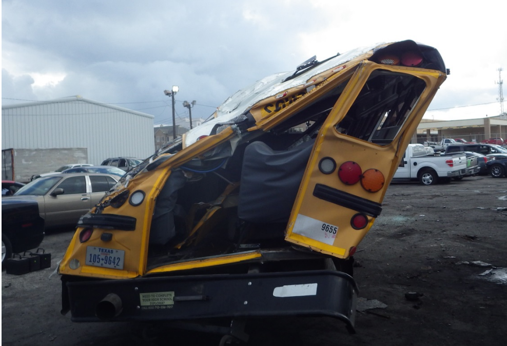
Figure 1. View showing contact damage to the top left corner of the HISD bus.
