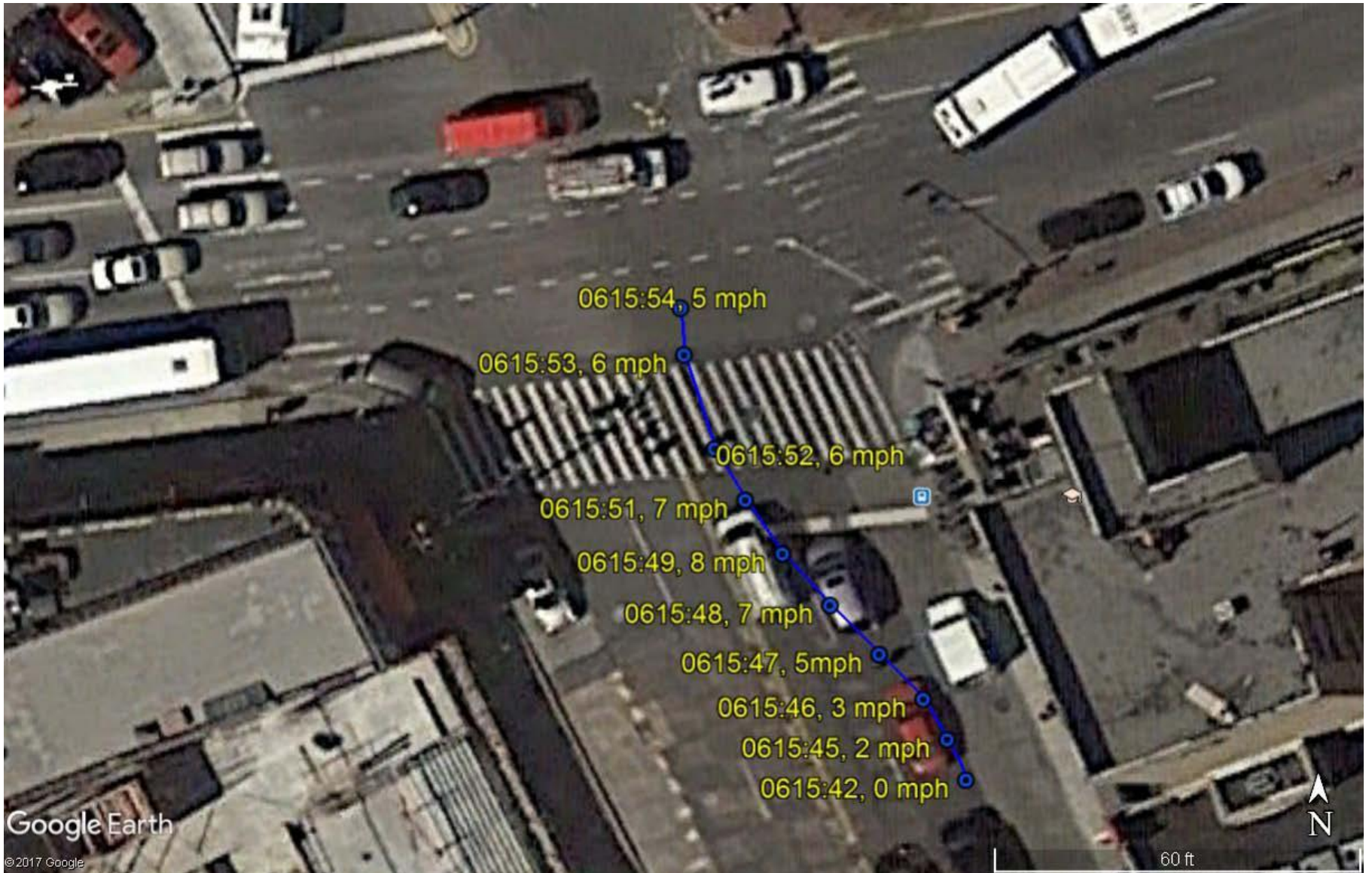
Figure 6. Google Earth overlay showing position of the MTA transit bus during the last seconds prior to the crash. Time is expressed in EDT.
