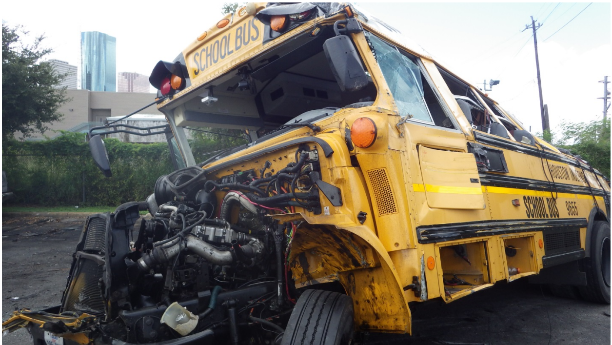
Vehicle Photo 1 – Overall view of the damage to the left side of the HISD school bus from the left front corner. Damage to the engine compartment, windshield and side windows can be seen.
