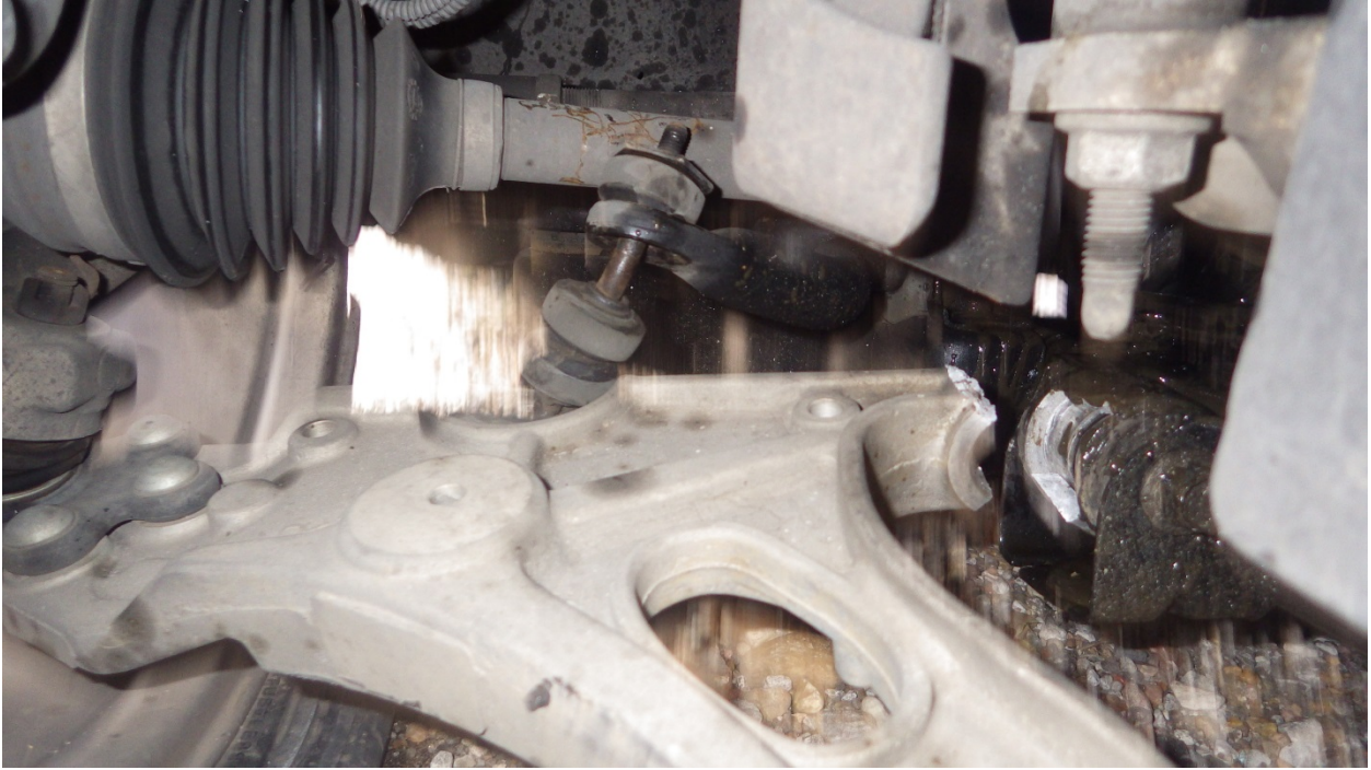
Vehicle Photo 3 – View showing the fractured Buick LeSabre passenger side control arm.
