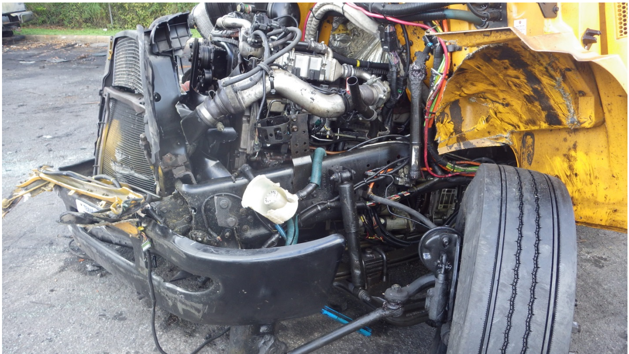
Vehicle Photo 2 – View showing damaged HISD school bus steering components.
