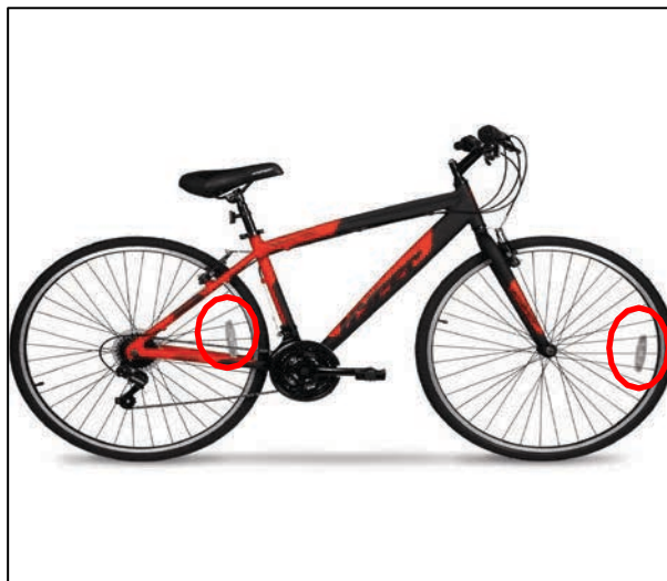
Figure 6 – Photo of exemplar Hyper 700c SpinFit Hybrid Bike showing reflectors mounted on front and rear wheels circled in red
