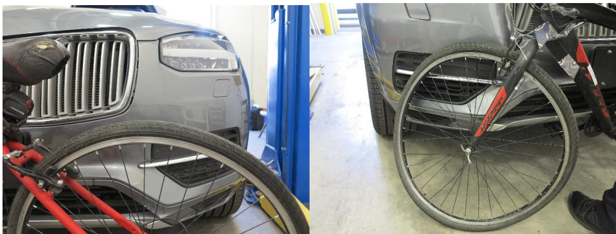
Figure 2 – Rear and front bicycle tire transfer print on front bumper cover
