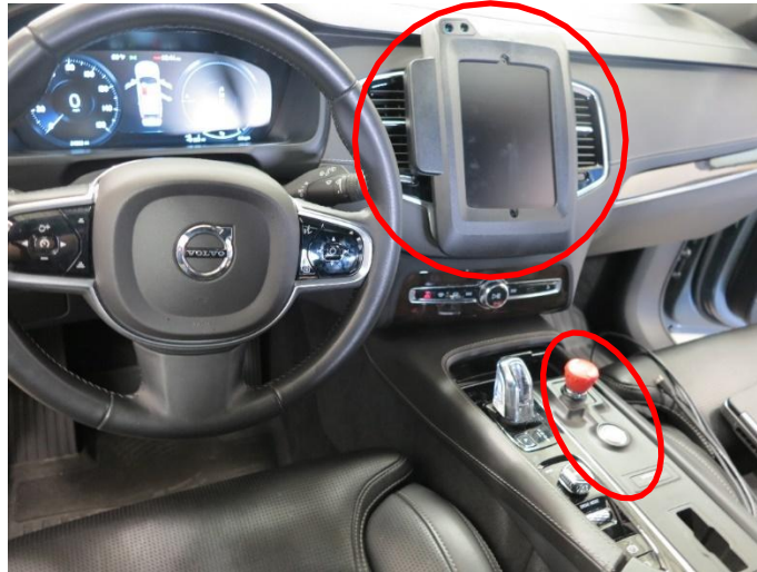
Figure 4 – Additional equipment added to the driver's compartment by Uber ATG, circled in red
