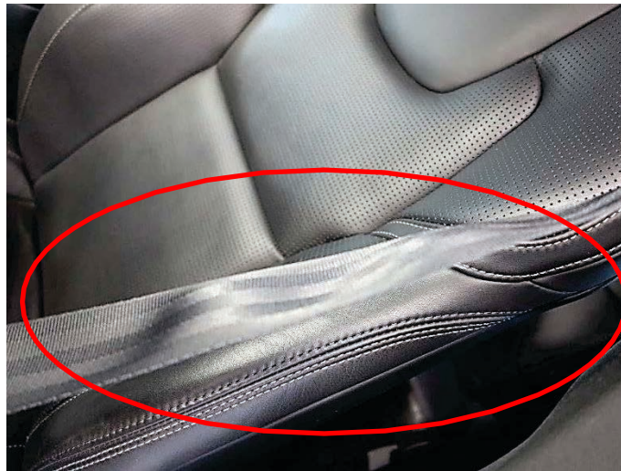
Figure 3 – Drivers seatbelt of the 2017 Volvo XC90 showing cupping, circled in red
