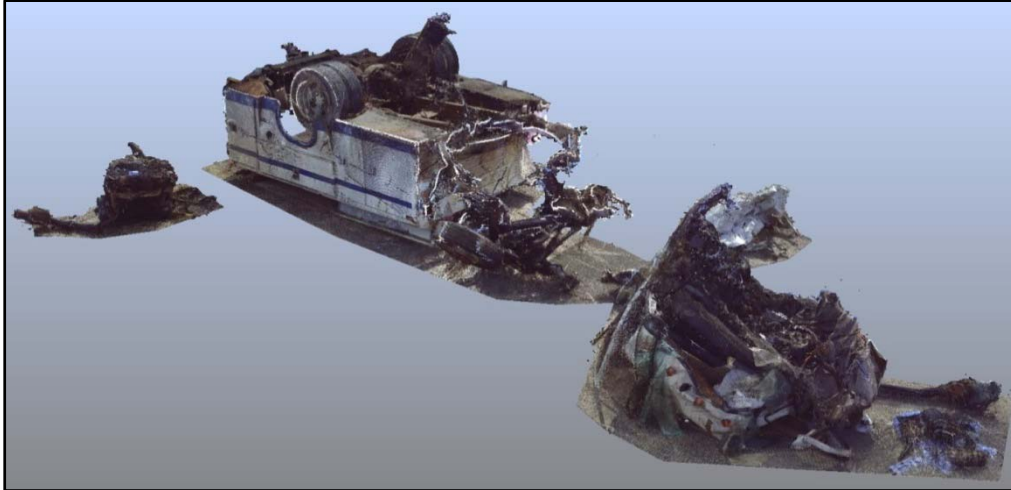
Figure 1: Image of 3-D Laser Scan of Ford F-450 Utility Truck
