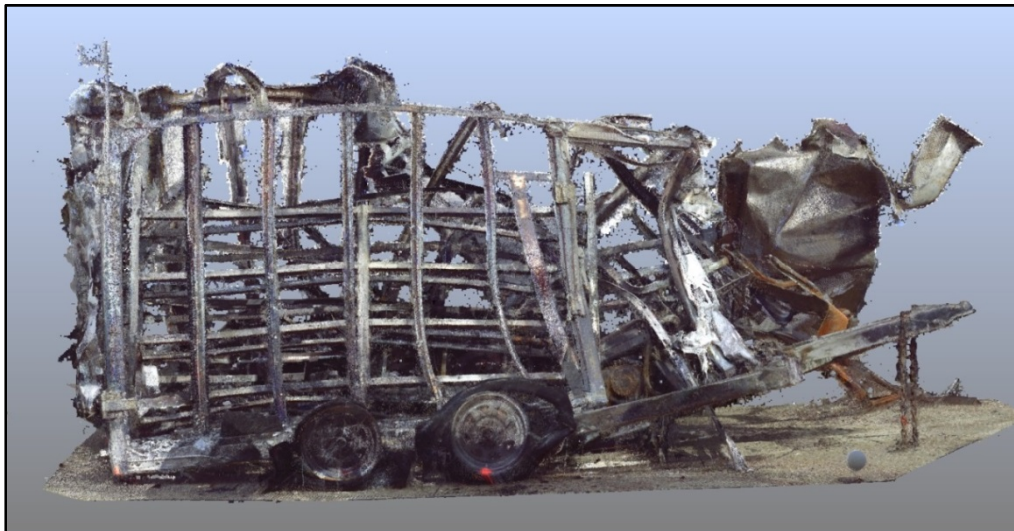
Figure 2: Image of 3-D Laser Scan of Wells Cargo Utility Trailer
