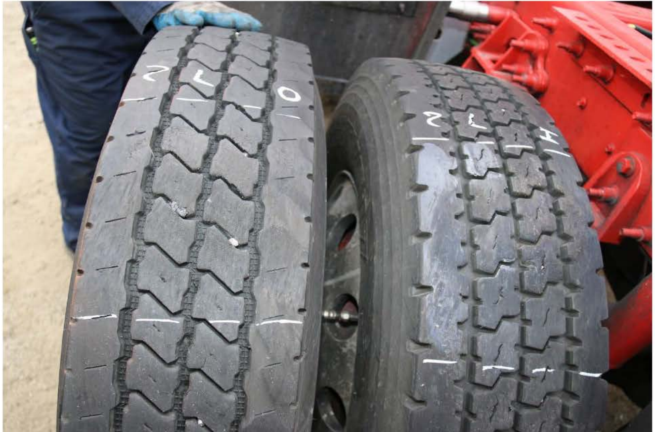
This is a view of the roadway abrasions on the tires on the left side of axle 2.
