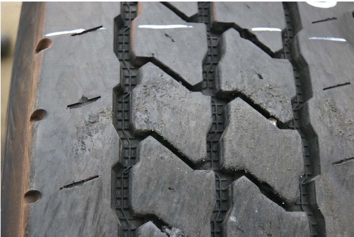
This is a close-up view of the roadway abrasion on one of the drive tires showing the balled up rubber and striations.
