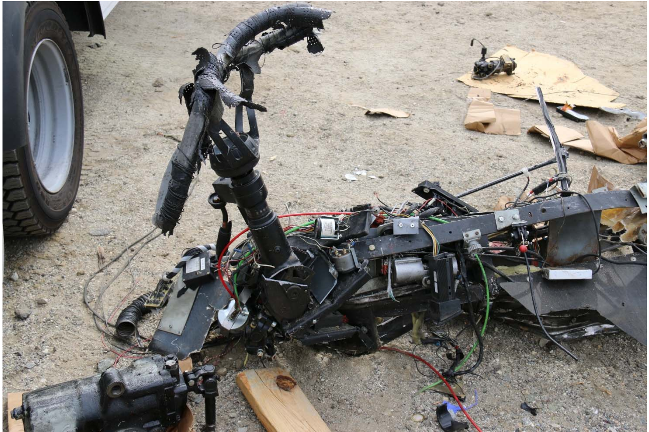
This is a view of the collapsed steering wheel ring, broken steering column, and what is left of the dash and instrument panel. The gauges and switches are either broken or missing
