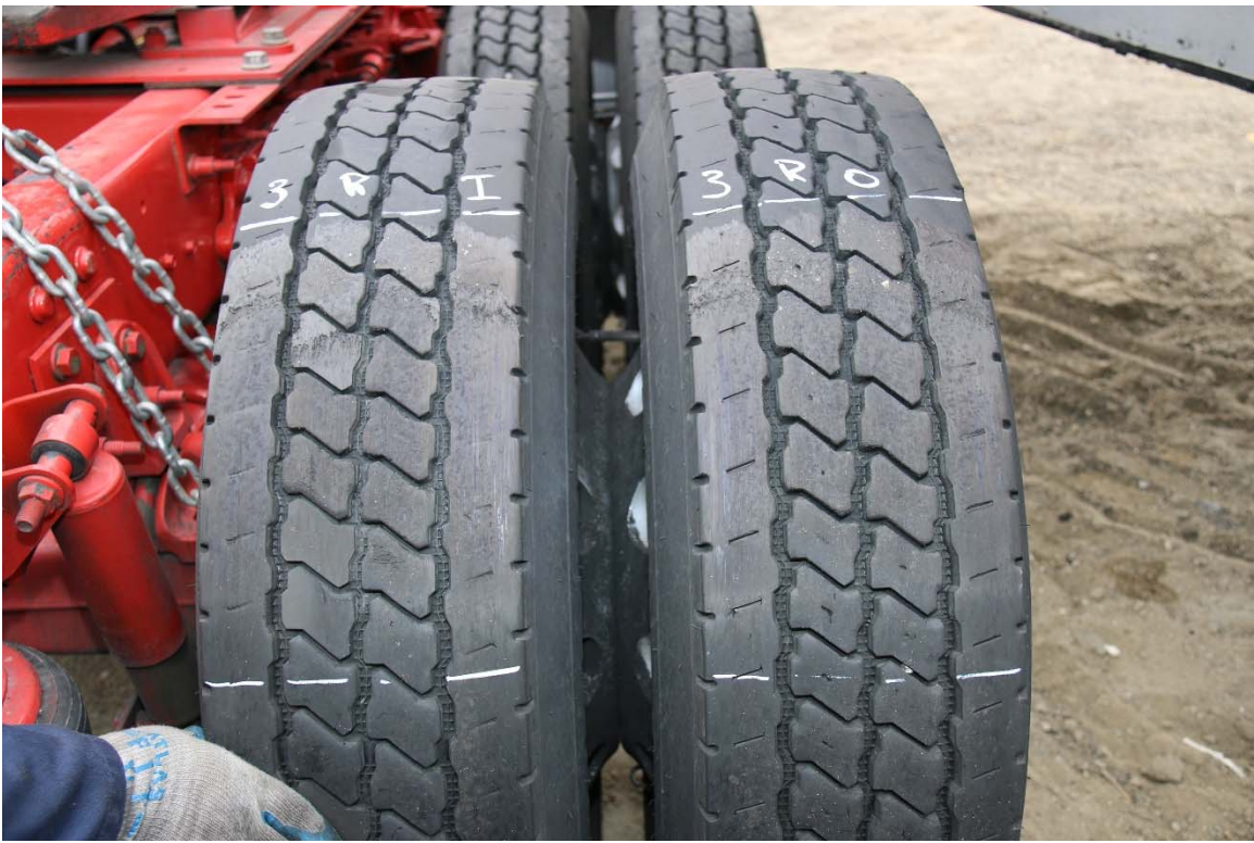
This is a view of the roadway abrasions on the tires on the right side of axle 3.
