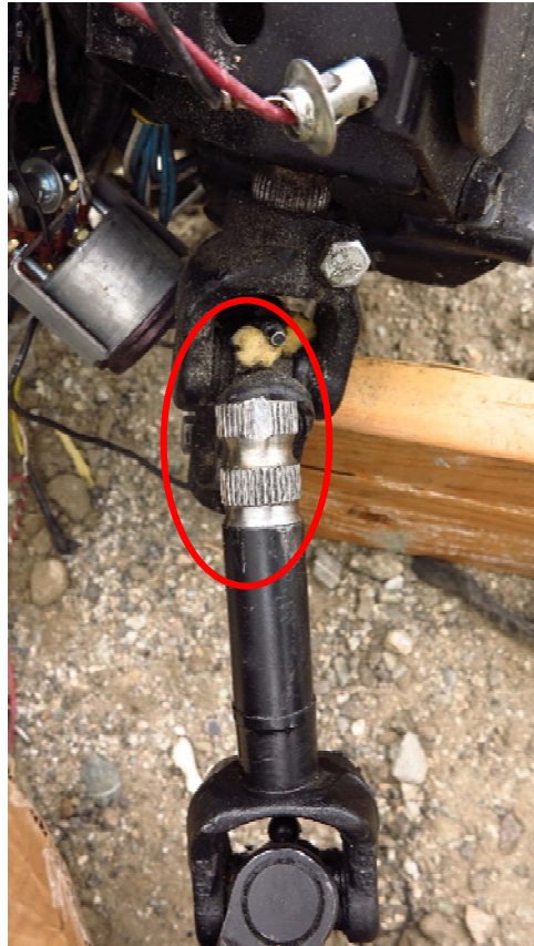
This is a view of the steering intermediate shaft. The red circle shows the damaged splines from having been pulled from the universal joint during the crash.
