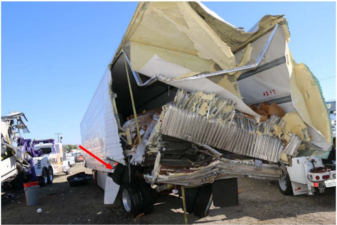
This view is looking from the left rear to the left front of the semitrailer. The rear of the semitrailer shows extensive crash damage. A portion of the left sidewall is missing. The red arrow is pointing to the left side of axle 5 tires which were displaced forward and on top of axle 4 tires. The cargo doors and frame are missing.
