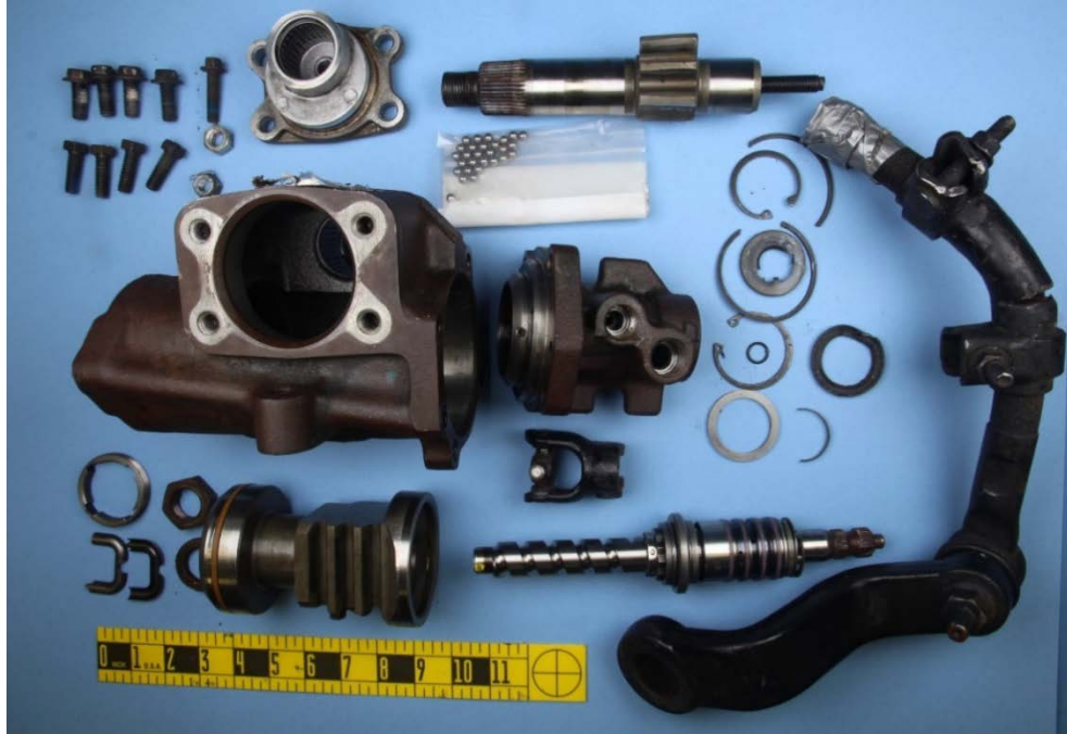
Figure 4 – Disassembled steering gearbox of the 2007 Dodge Ram 3500 pickup truck
