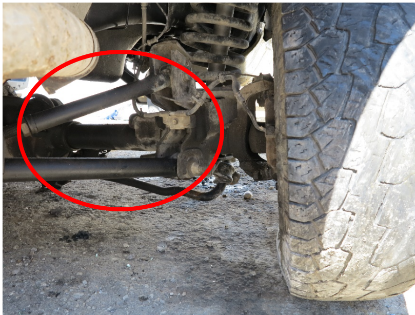
Figure 6 – Right-side aftermarket adjustable control arms (circled in red) of the 2007 Dodge Ram 3500 pickup truck
