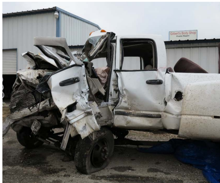
Figure 2 – Left-side view of the 2007 Dodge Ram 3500 pickup truck showing contact and induced damage to the left side of the vehicle
