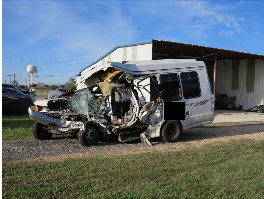
Figure 8 - Left side view of the 2004 Turtle Top bus showing the front and left side contact and induced damage
