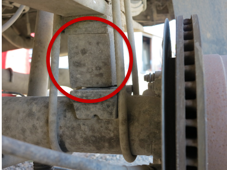
Figure 7 - Left-side aftermarket 4-Inch lift block (circled in red) on rear axle of the 2007 Dodge Ram 3500 pickup truck
