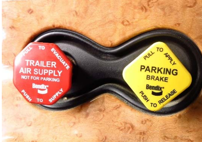
Figure 3: Truck Tractor Push-Pull Valve Brake Knobs
