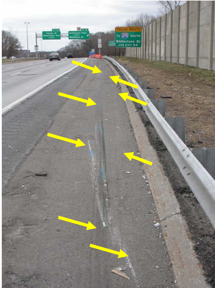
Figure 3 – After initially striking the guardrail the bus veered away from the guardrail and lost contact the guard rail for short distance. The arrows shown in the photograph indicate evidence of the path of the bus during the time it lost contact with the guardrail. Note that there is no evidence of contact damage from the bus visible on the guardrail. (Unless indicated by an arrow, tiremarks and scrapemarks shown in the photograph are not associated with this accident.)
