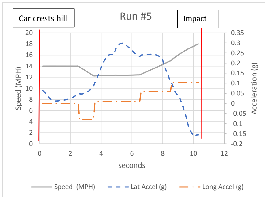
Figure 5 – Plot diagram of the truck’s speed and acceleration versus time for simulation Run #5.
