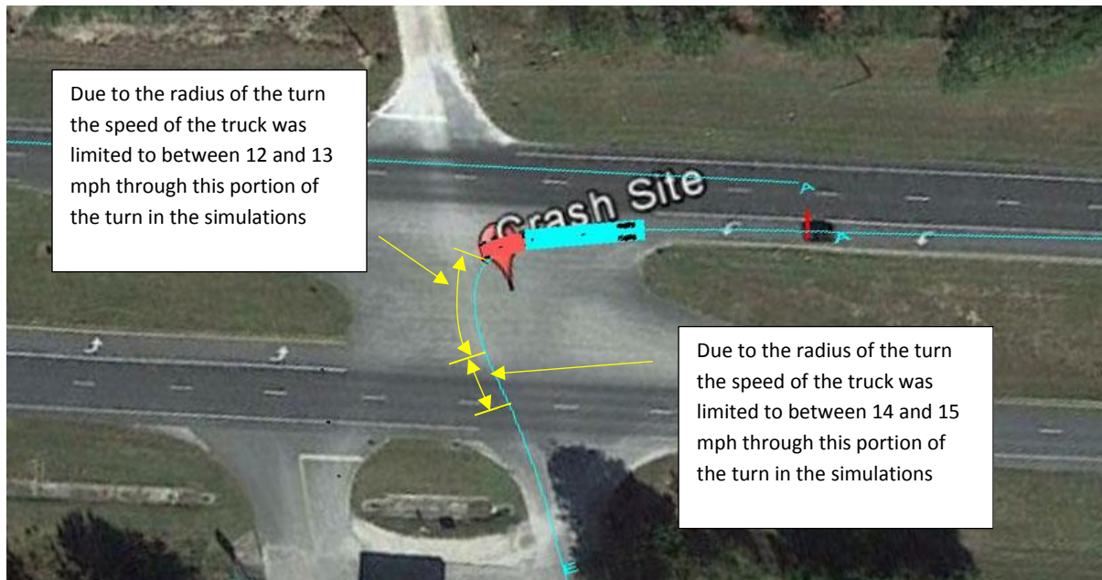
Figure 3 - Due to the radius the turn the speed of the truck was limited through portions of the curve. The truck's maximum speeds through portions of the turn are noted in the figure.
