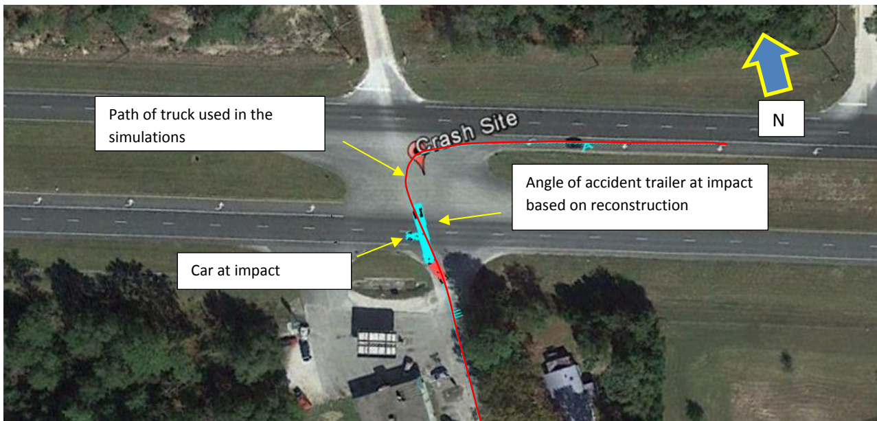
Figure 1 – The red line indicates the path of the truck used in the study. The angle of the trailer shown in figure is the approximate angle of the accident trailer at impact based on the damages to the trailer.
