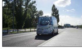
directly with a plug. The vehicle is equipped with the latest generation in sensors to enable it to find its way around and navigate effectively. Thanks to this technology, the NAVYA ARMA is able to position itself within a few centimetres from the desired target and to identify all types of obstacle on the road (fixed such as posts or mobile such as pedestrians) or signage in both daylight and at night time.
