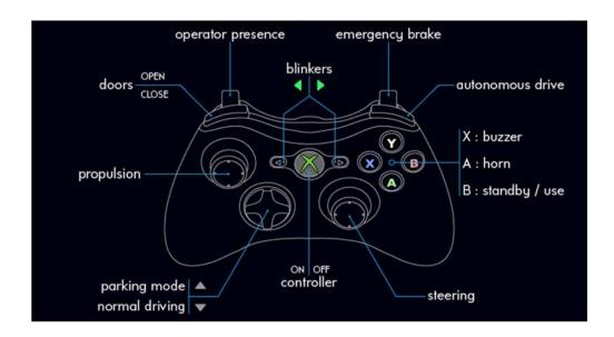
This is a complete list of the features of the controller for manual driving.
