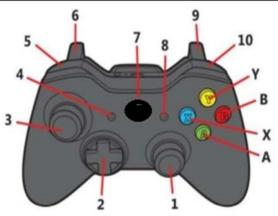
**Direction**: To steer the vehicle, gradually orient the steering joystick (1) to the left (or right) to turn left (or right) in the forward direction.
