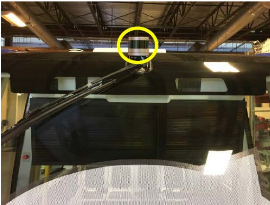
Figure 2. The location of a lidar on the roof of the shuttle. Another lidar is positioned at the same location at the rear of the shuttle.
