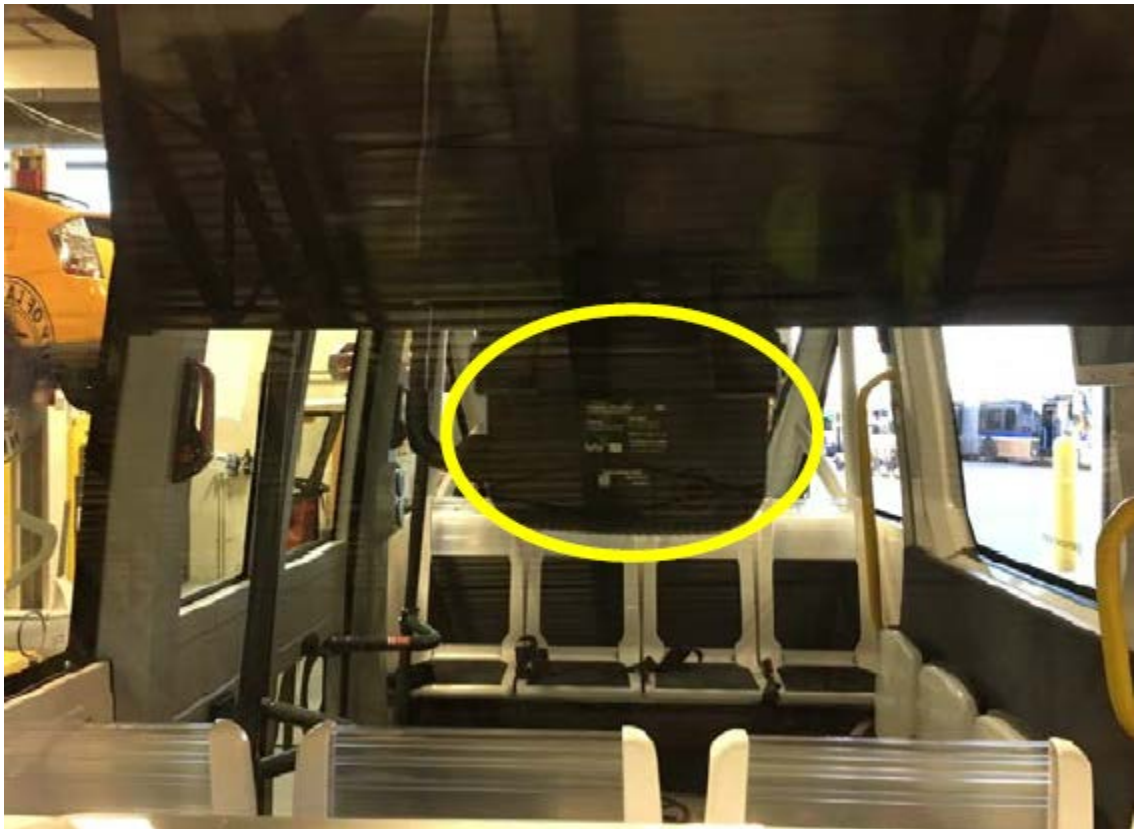
Figure 6. The location of Lytx DriveCam on the windshield in front of the shuttle.
