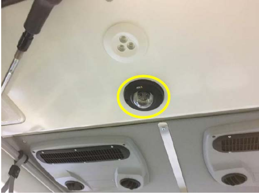
Figure 5. The location of the fish-eye camera inside the shuttle.
