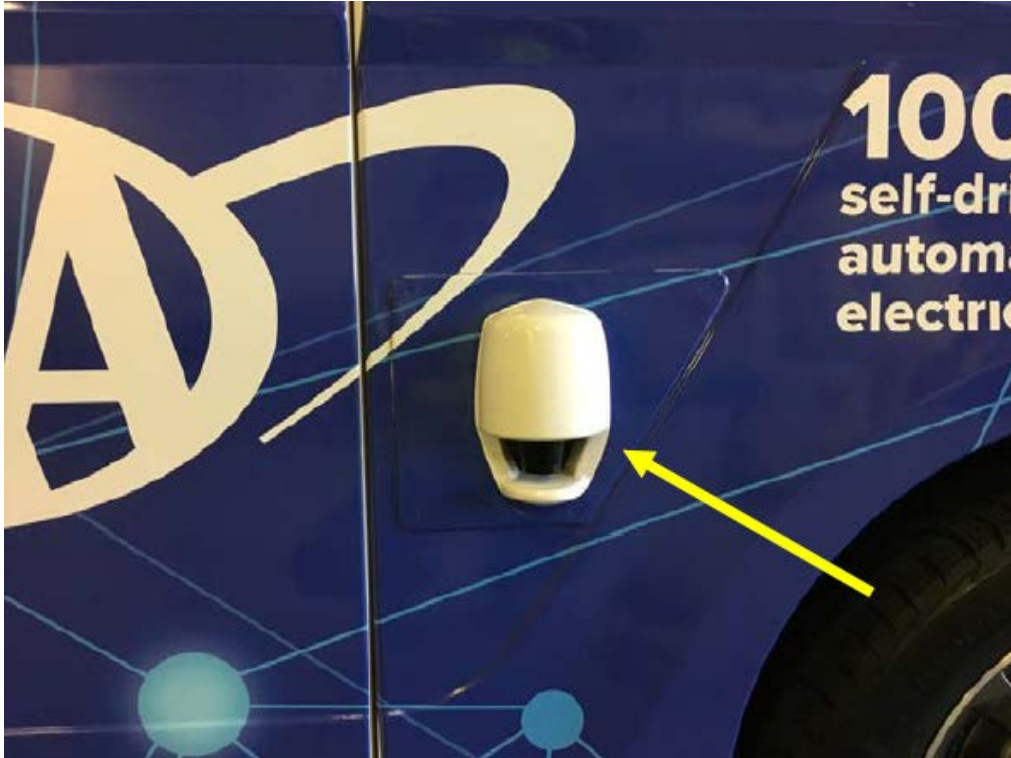
Figure 3. The location of a lidar on the left side of the shuttle. Another lidar is positioned at the same location on the right side.
