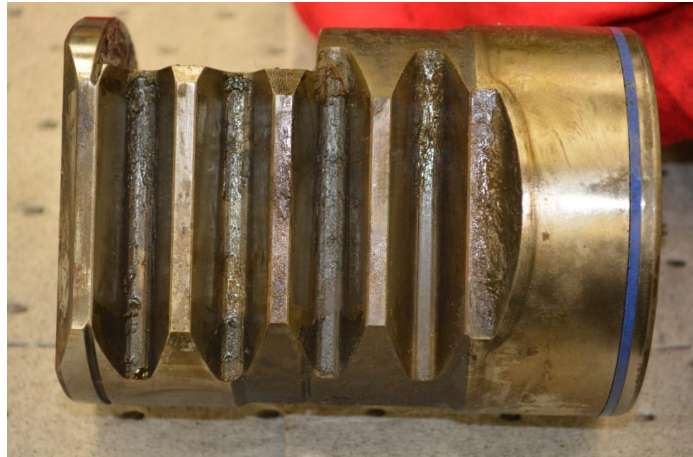
Rack Piston, dirty, but no damage
