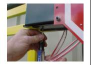
2. Use a screwdriver (or similar tool) to tap the cam shaft back up inside the unit.
