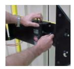
4. Remove screws from both ends of the cover using 5/16" socket.
