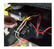
16. Install new 005150 module into position as shown above. Timing mark MUST be facing toward the direction of the blade. (Ex. If blade is fully extended, timing mark must be turned to front of unit). Push module shaft through lower hinge hole. Fasten with (2) 11/32" hex nuts from original micro switch assy.
