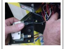
10. Remove all wires from micro switch assembly. Black heater wire remains with assy.
