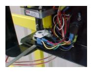
9. Using a flat blade screwdriver, carefully pry the micro switch plate upwards. CAUTION-bushing may break and snap ring will make a loud noise when released. Discard the snap ring and bushing.
