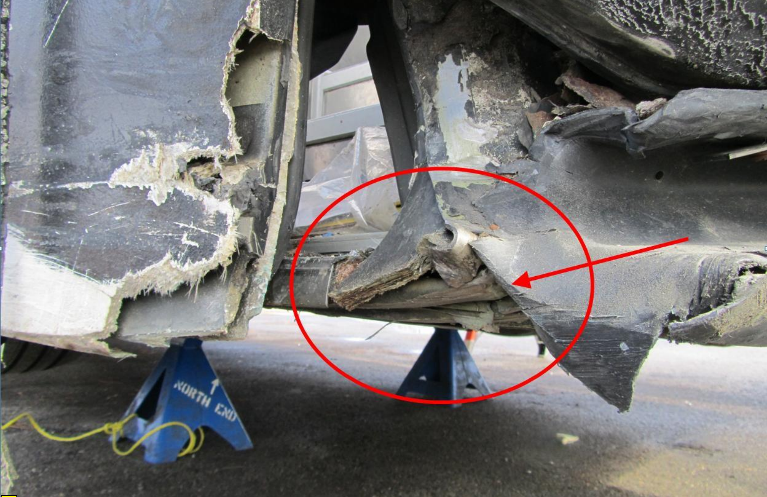
Photo 5 - Right front lower edge of the bus body, showing scrape marks
