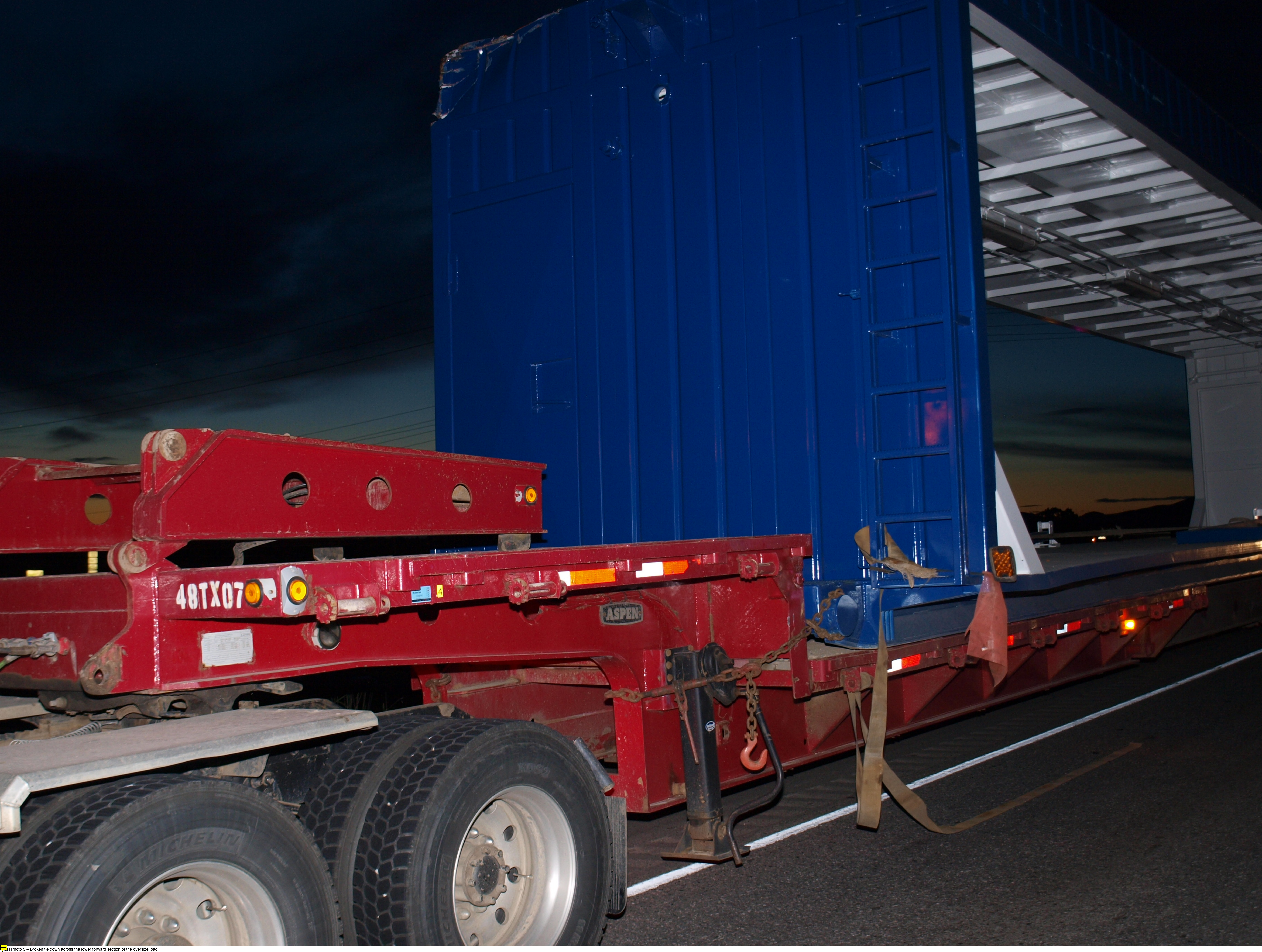
Photo 5 - Broken tie down across the lower forward section of the oversize load
