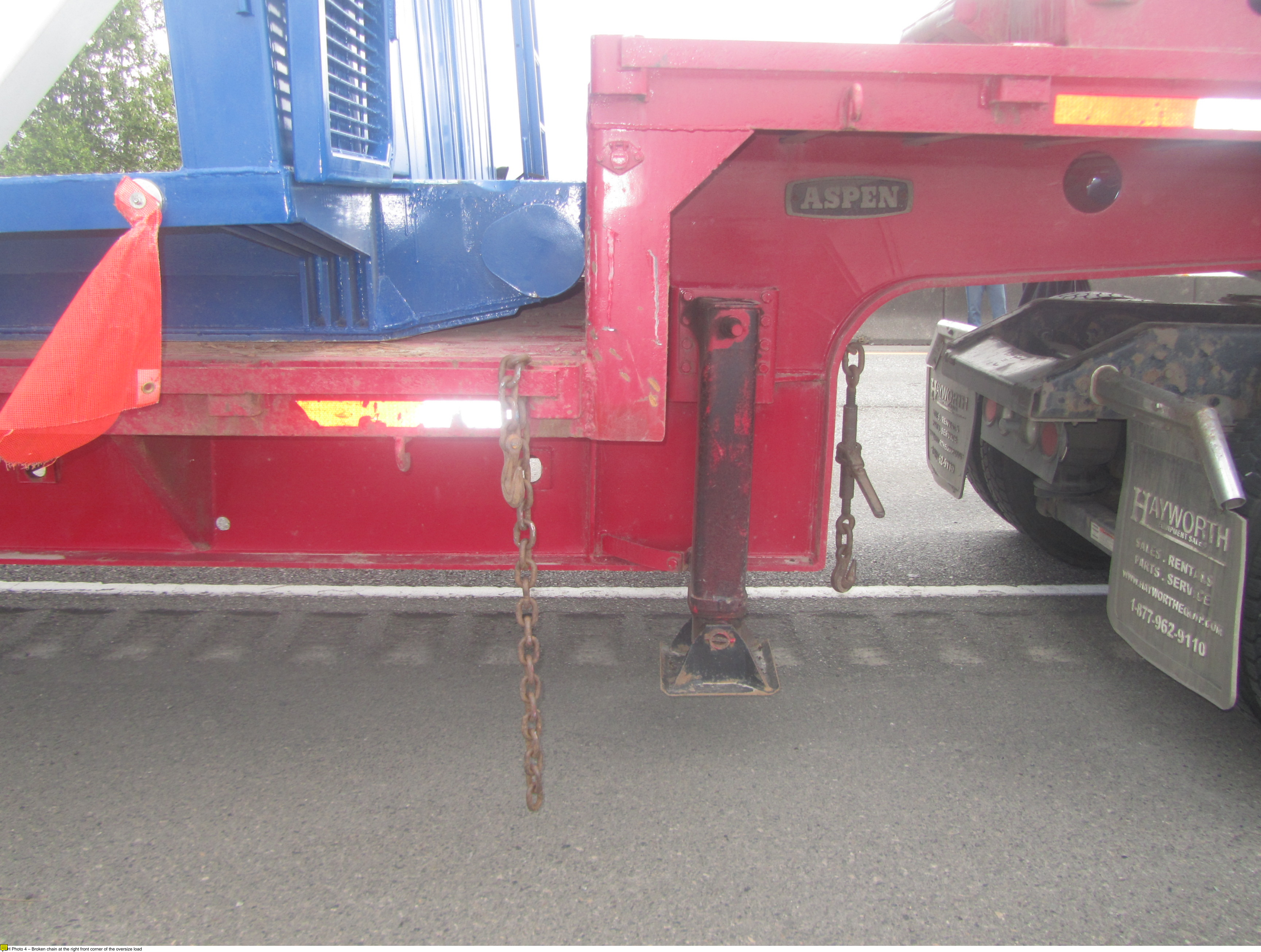
Photo 4 - Broken chain at the right front corner of the oversized load
