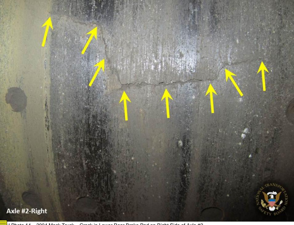
H Photo 14 – 2004 Mack Truck – Crack in Lower Rear Brake Pad on Right Side of Axle #2
