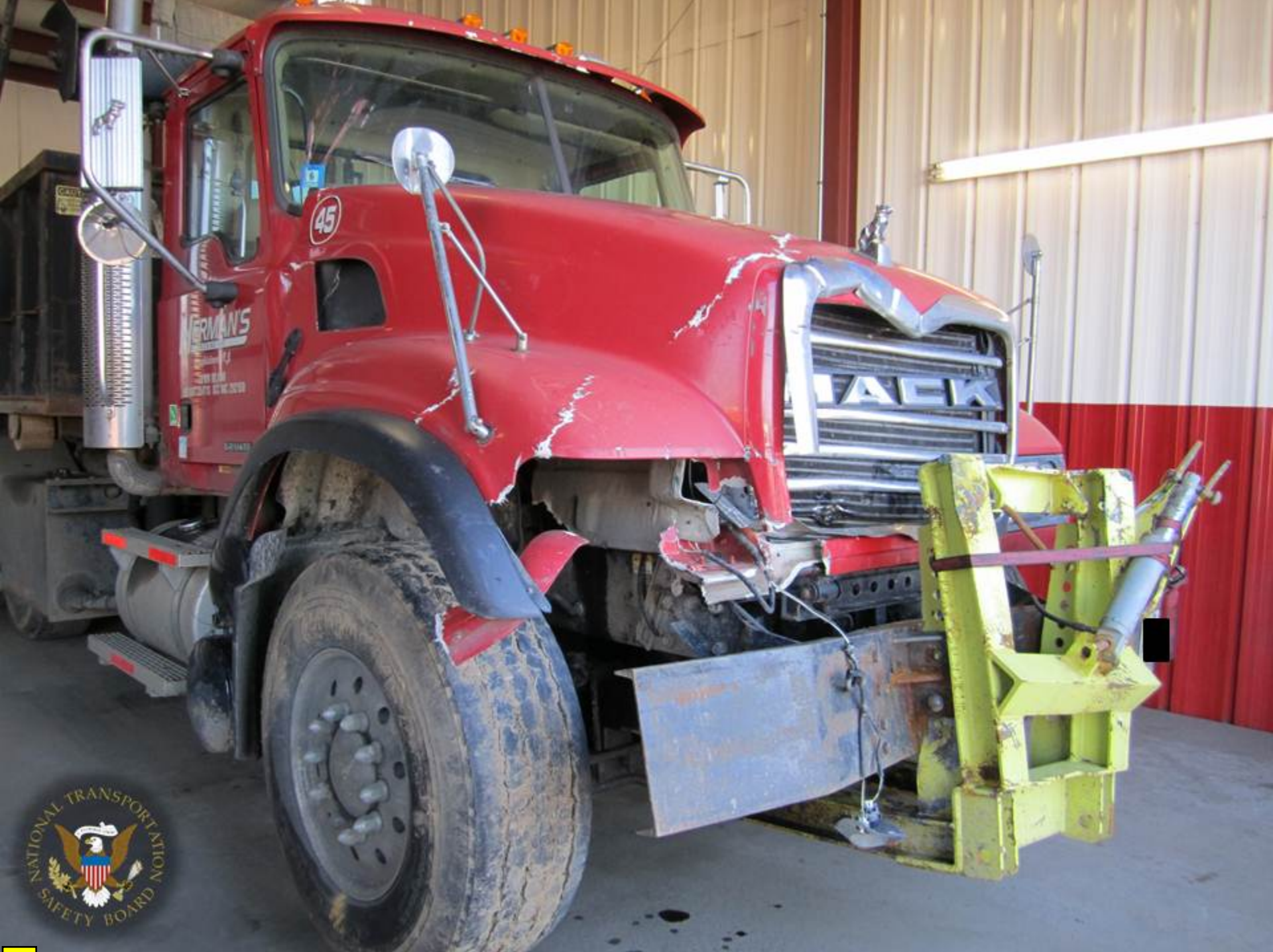
Photo 08 – 2004 Mack Truck – Contact Damage to Front
