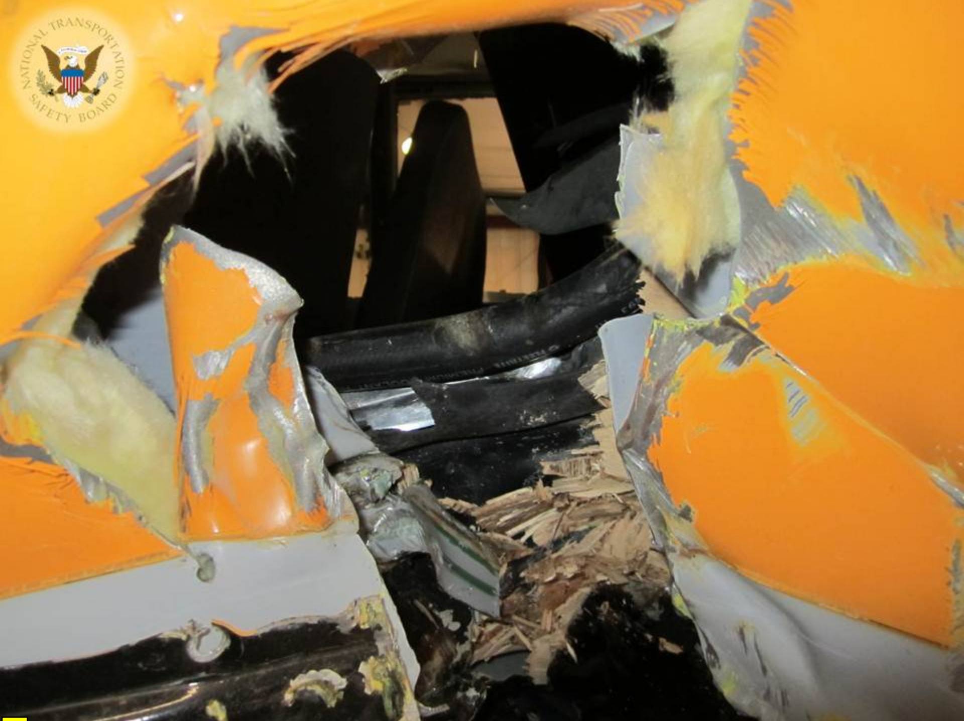
Photo 02 – 2012 IC School Bus – Penetrating Damage to Rear Left Side
