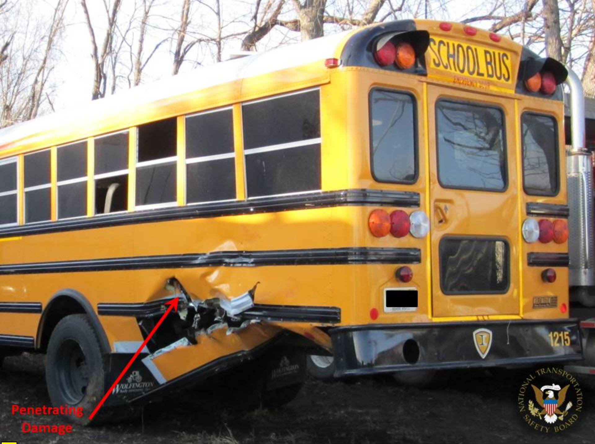
Photo 01 - 2012 IC School Bus – Contact Damage to Rear Left Side
