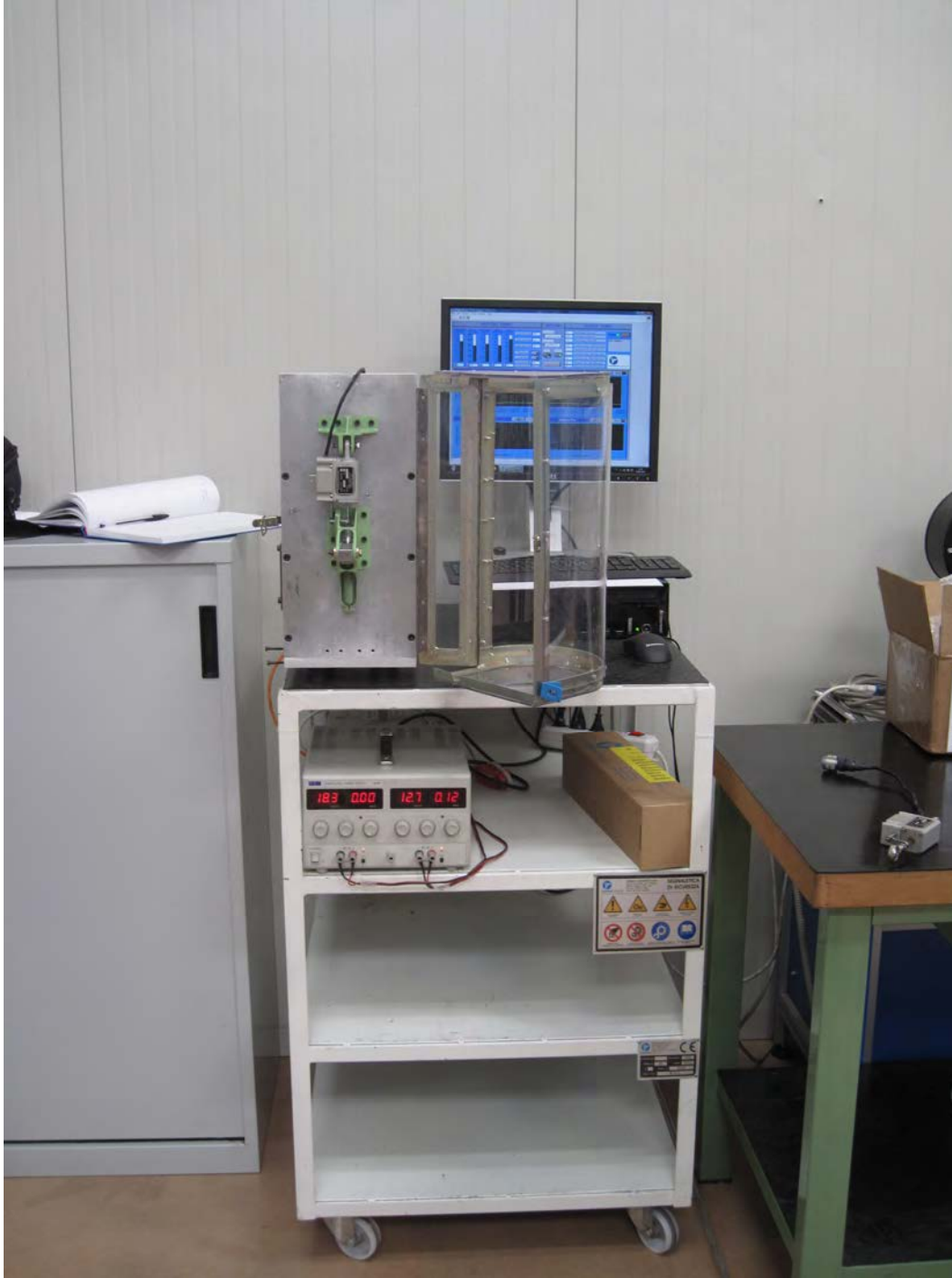
Photo 2 Gust Lock Test Rig (a new Actuator is installed)
