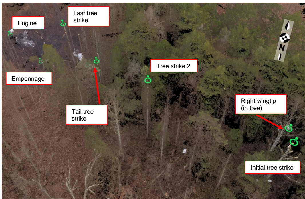
Figure 5 – 3D Point Cloud showing intermediate tree strike witness marks
