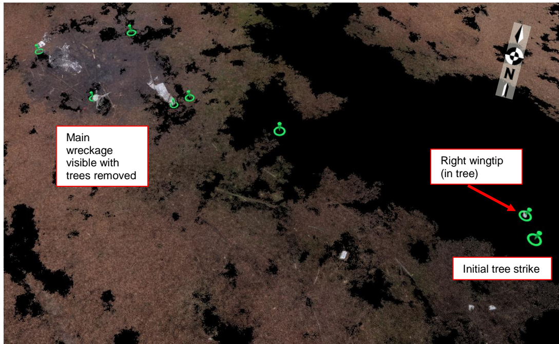
Figure 6 – 3D Point Cloud with “high vegetation” classification removed
