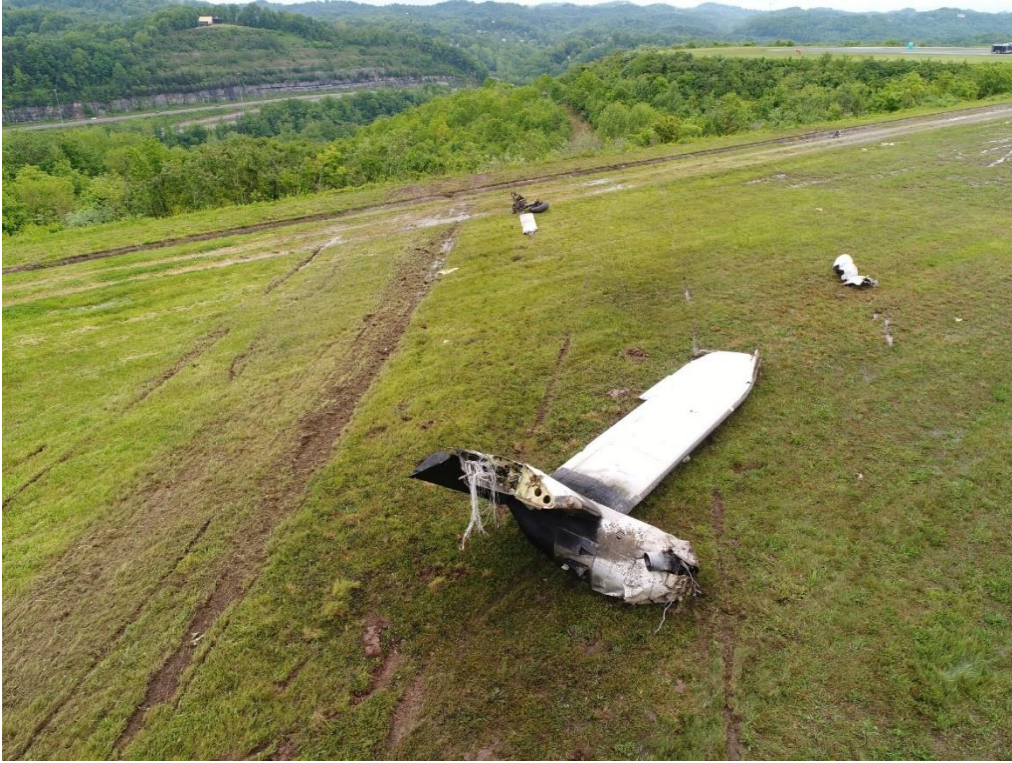
Figure 3 - Photo Left Wing and Witness Mark
