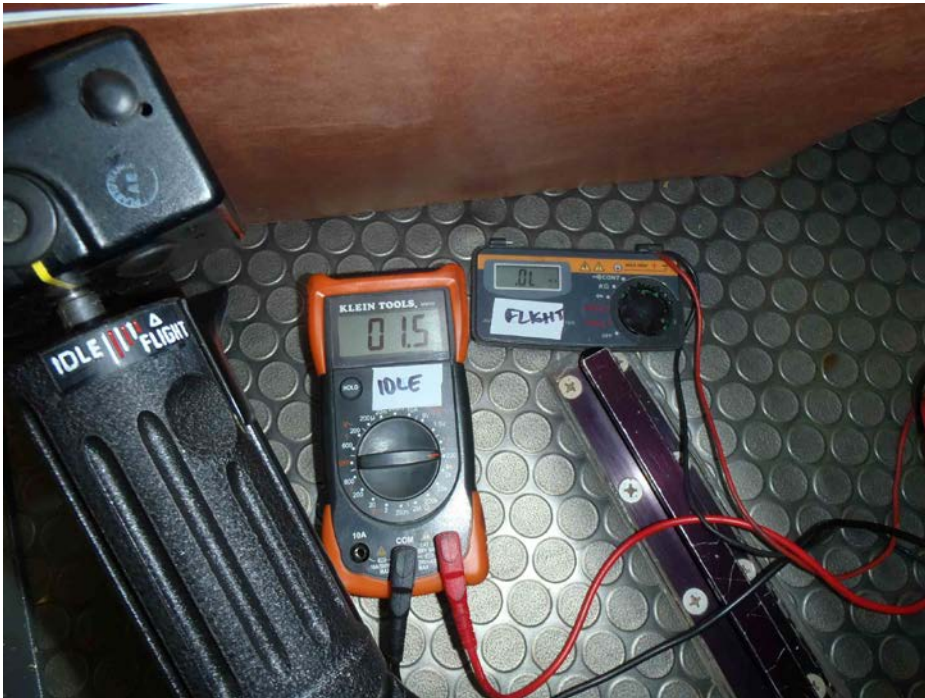
Photo 2 - Resistance at IDLE
