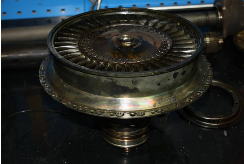
Figure 5: Power turbine - removed during wreckage recovery
