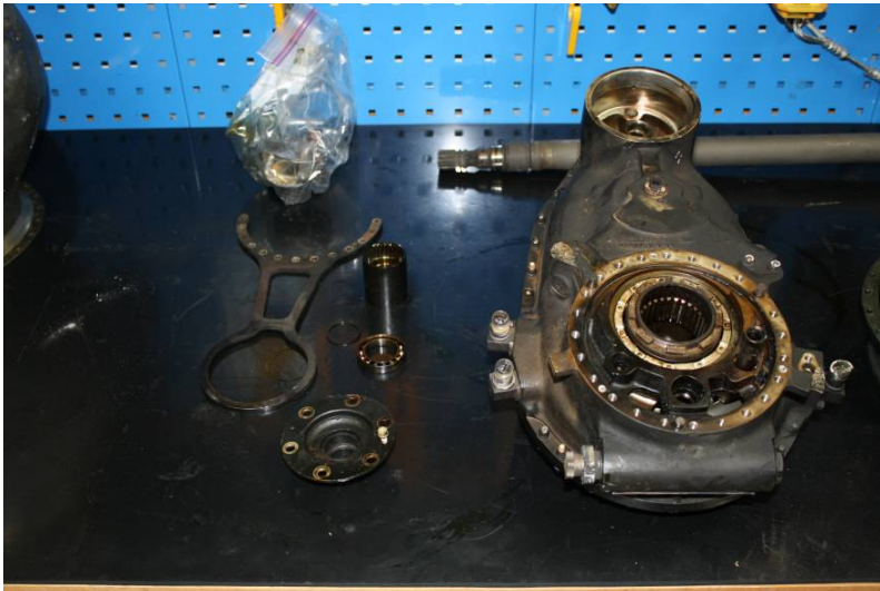
Figure 4: Reduction gearbox (MO5) - removed during wreckage recovery
