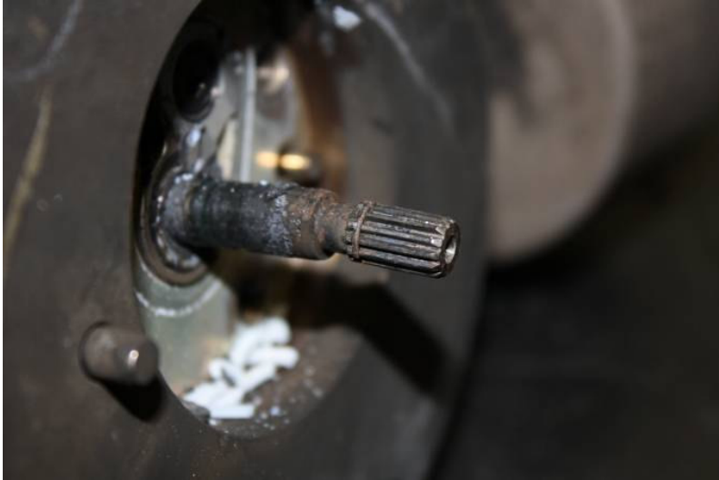
Figure 13 HMU shaft damage
