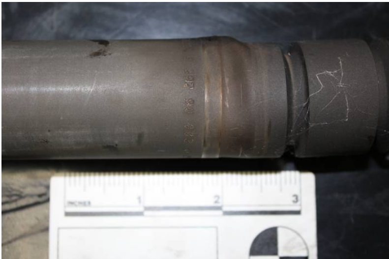
Figure 6 Free Wheel Shaft – torsional deformation
