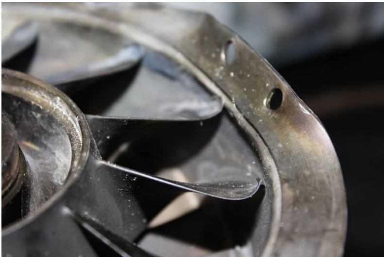
Figure 8 Axial compressor blades
