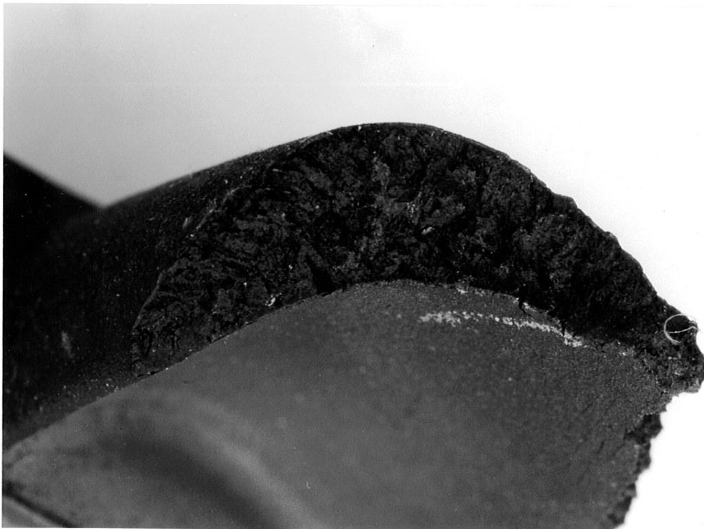
Figure 4 Close up view of a typical blade fracture surface showing an interdendritic fracture from applied overloads.
