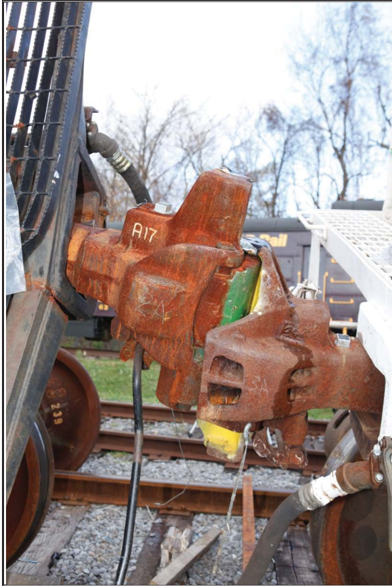
Figure 115: Final position of modified rotary coupler.
