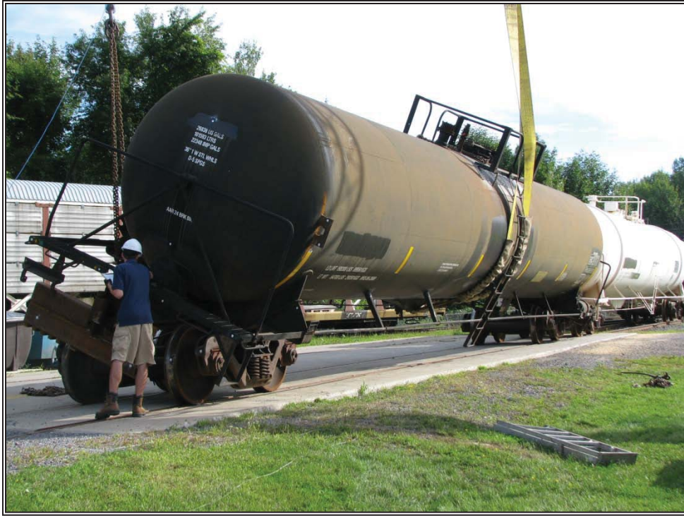
Figure 35: Pulling vertically at the end of the car from jacking pad.
