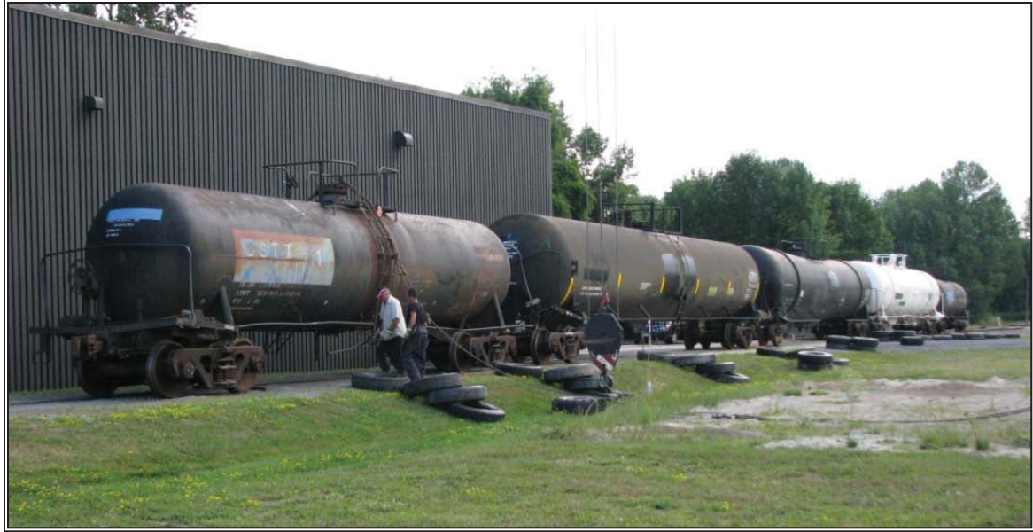
Figure 91: Test #3, dynamic testing with one modified rotary coupler and 5 tank cars - test setup.
