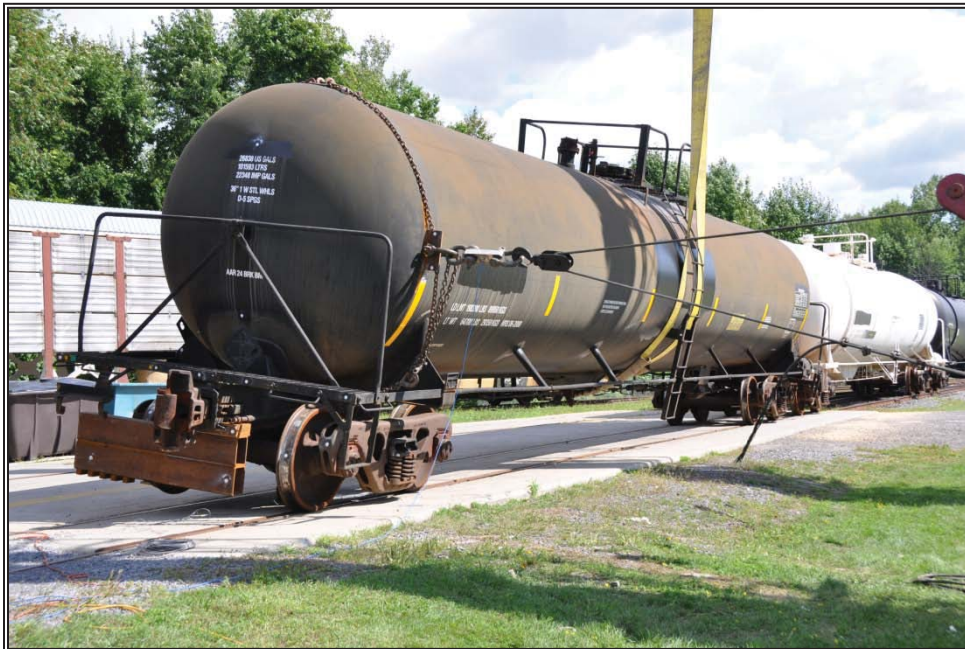
Figure 32: Pulling laterally at the end of the car from centre.
