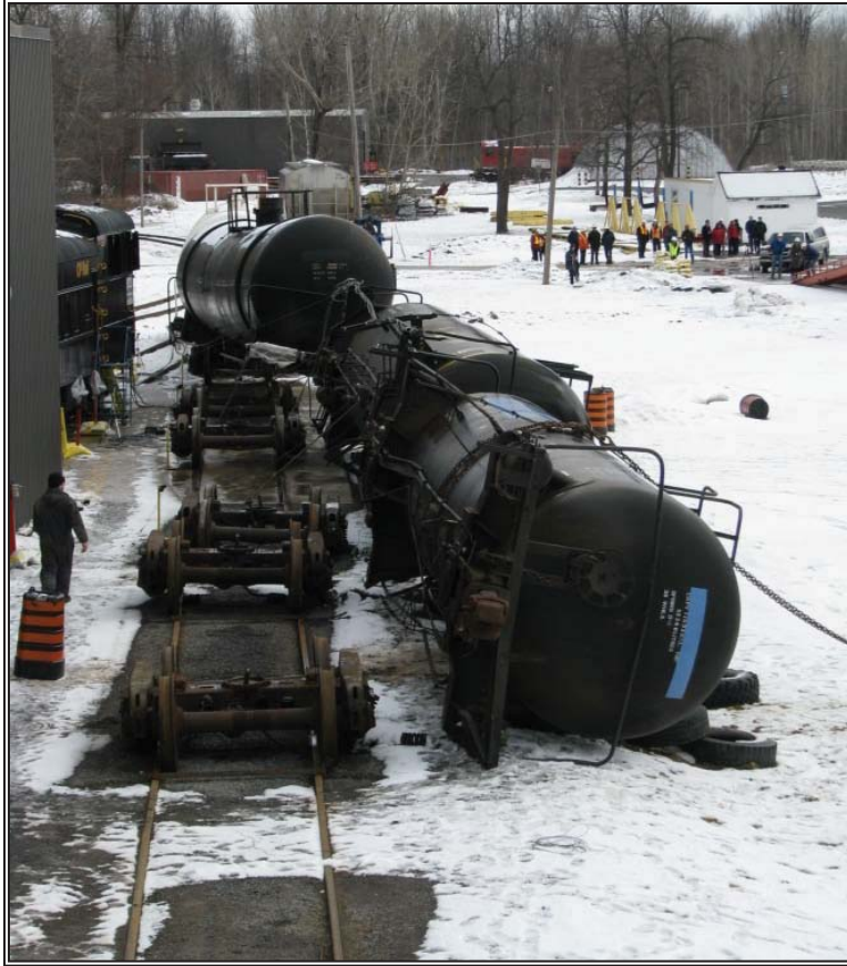
Figure 77: Test #2, cars after test, initiating end – rotary coupler stopped the rollover propagation.
