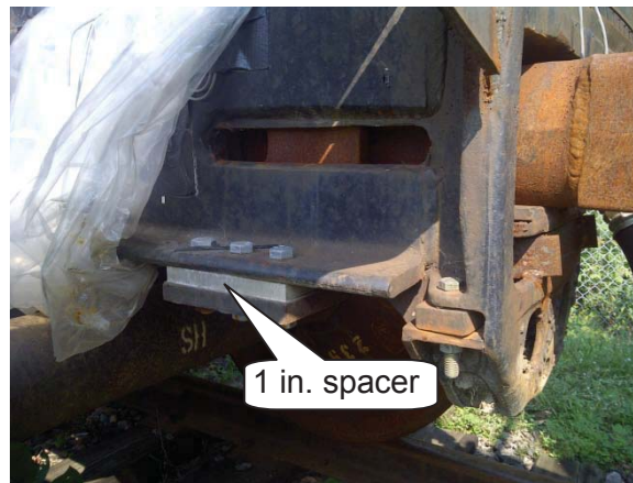
Figure 146: Insertion of 1 in. spacer below the yoke
