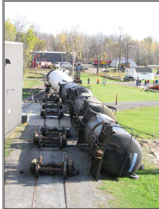
Figure 111: Test #4, dynamic testing with one modified rotary coupler and five tank cars.
