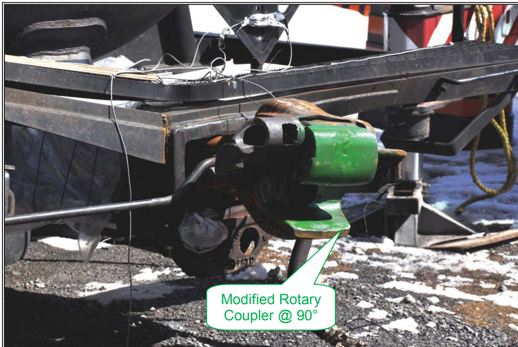
Figure 82: Test #2, rotary coupler orientation after test.
