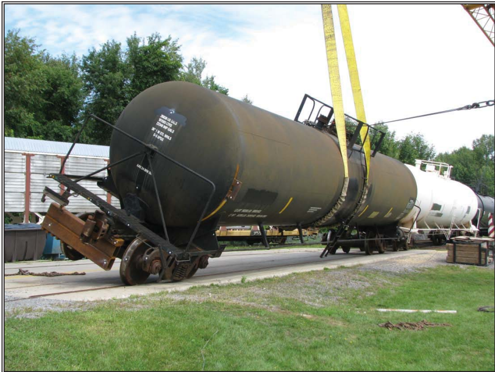
Figure 34: Pulling laterally at the middle of the car from top.
