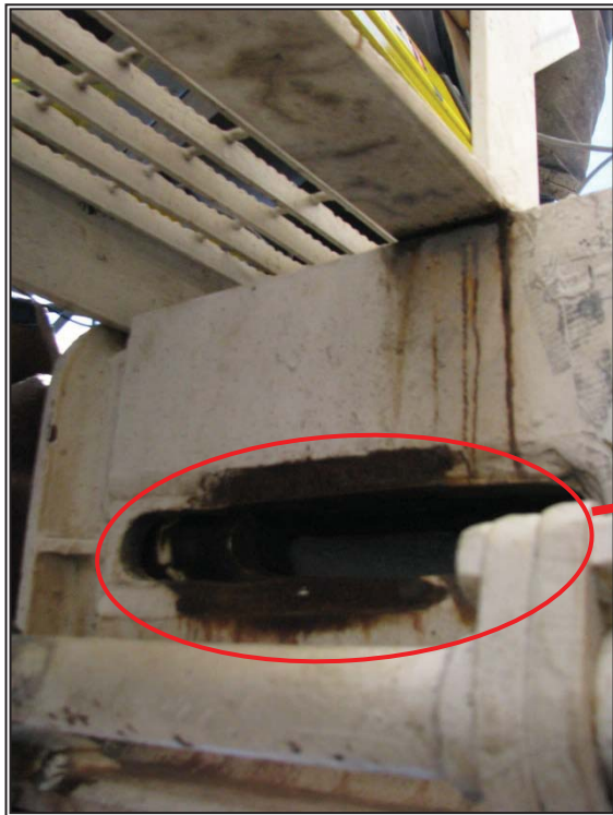
Figure 59: Test #1, broken coupler key of Car #II A-end.
