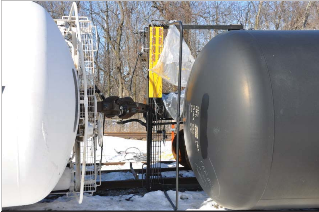
Figure 58: Test #1, cars after test – linked coupler.
