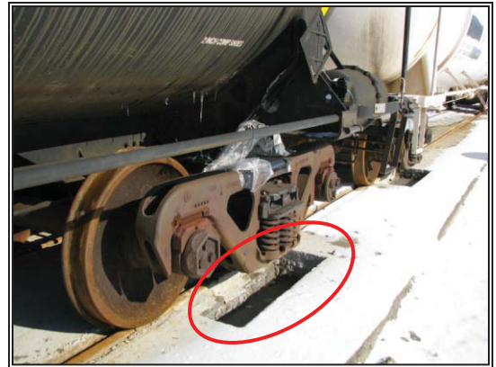
Figure 37: Truck almost touching the concrete during the dry-run test (left); and holes in the concrete during testing (right).
