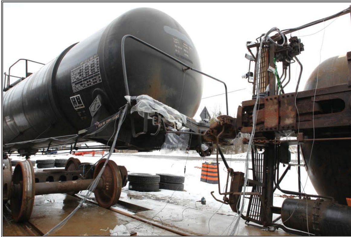
Figure 79: Test #2, cars after test, north side – modified rotary coupler junction.
