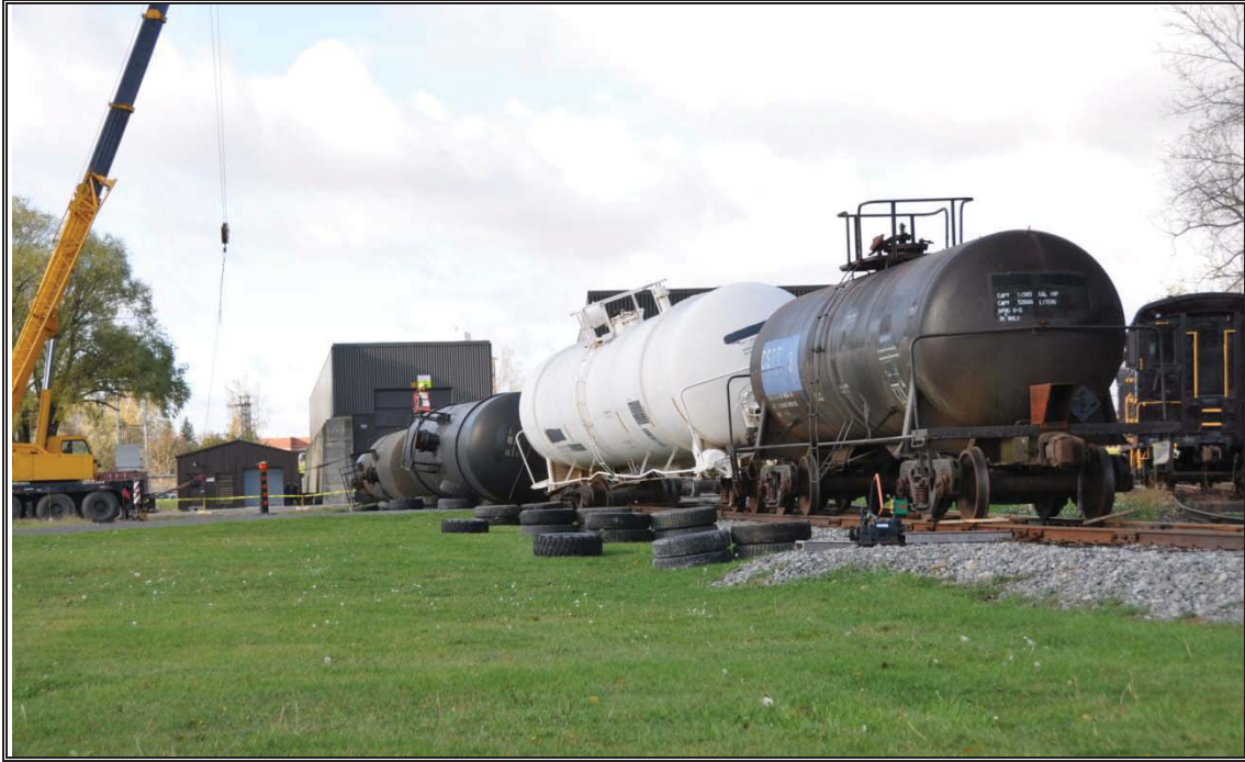
Figure 110: Test #4, five car test consist after rollover – rotary coupler stopped the rollover.
