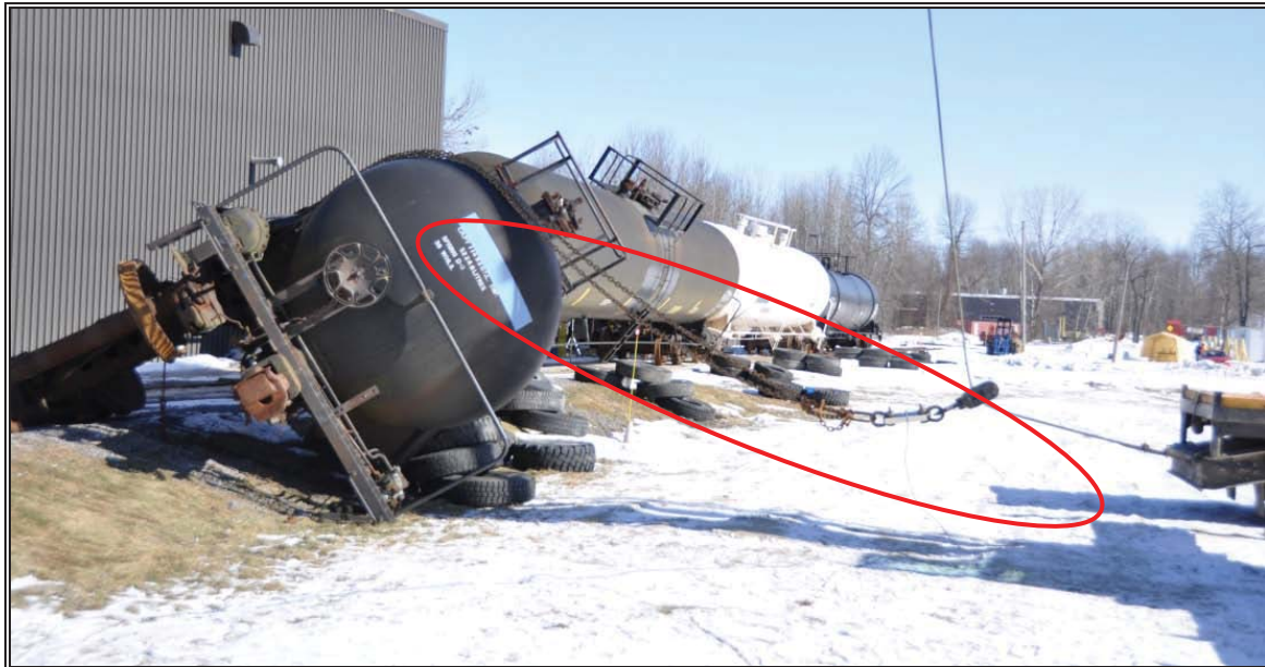
Figure 52: Test #1, initiating car on ground, failed rollover attempt.
