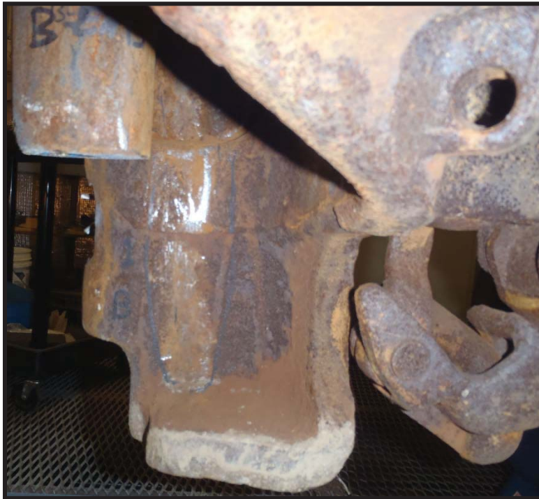
Figure 62: Gouge on wall of far end coupler of Car #I after Test #1.
