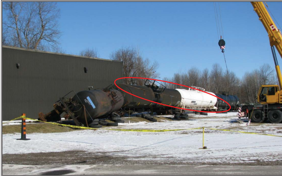
Figure 53: Test #1, pulling laterally at the near end of Car #1 from top.
