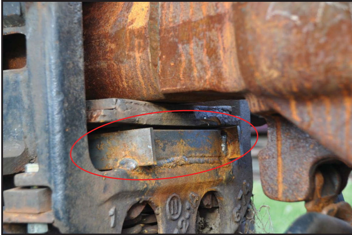
Figure 108: Rotary coupler with isolated carrier system.
