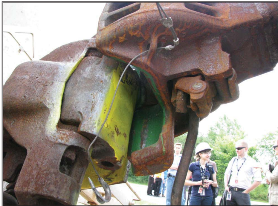
Figure 96: Test #3, rotary coupler partially opened after test.
