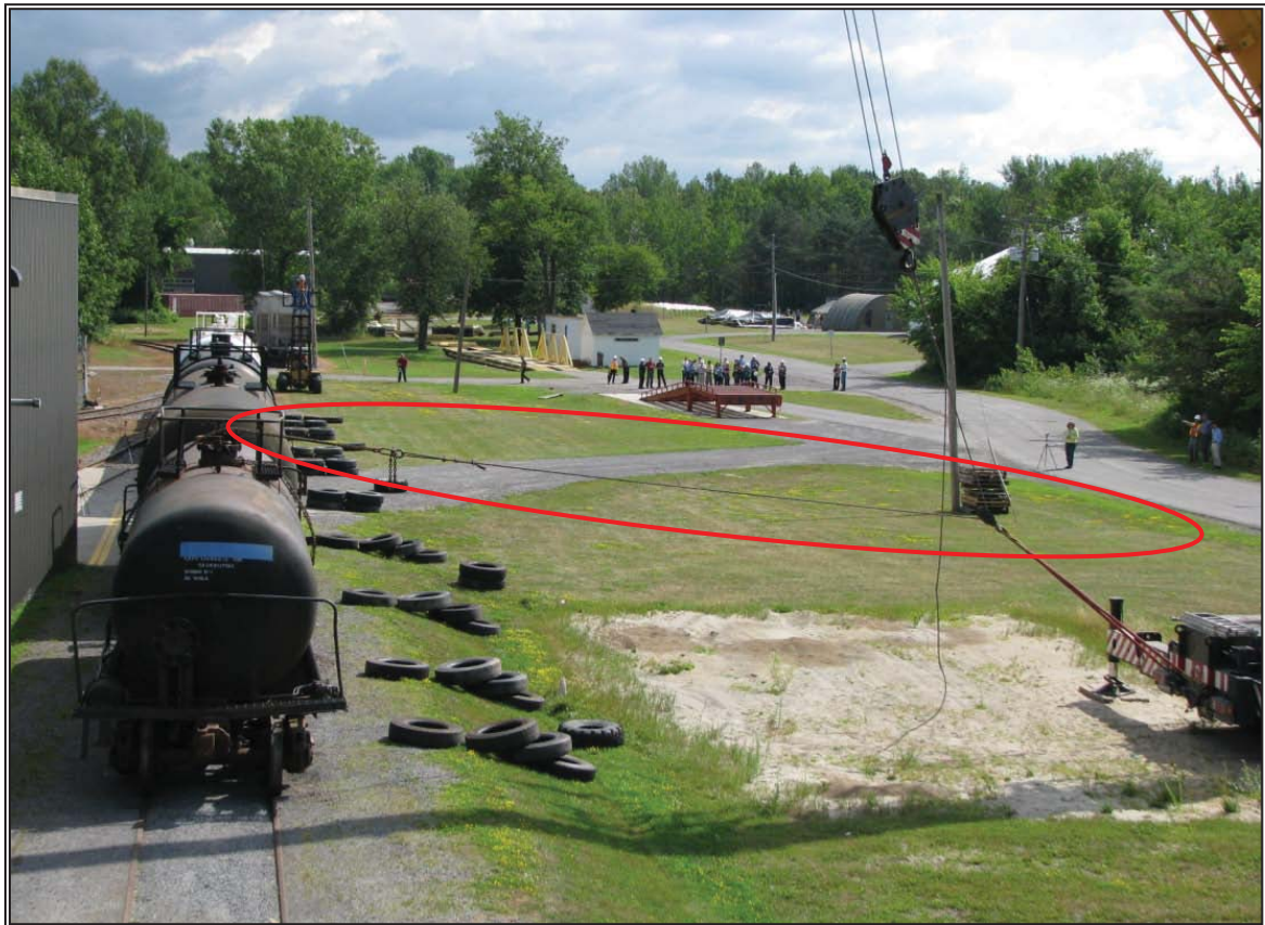
Figure 92: Test #3, lateral force applied at the middle of the initiating car from the top.
