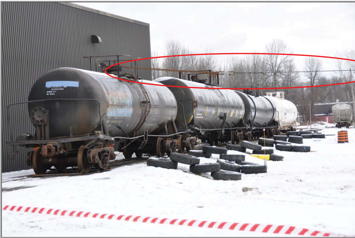
Figure 76: Test #2, dynamic testing with one modified rotary coupler and 4 tank cars - test setup.
