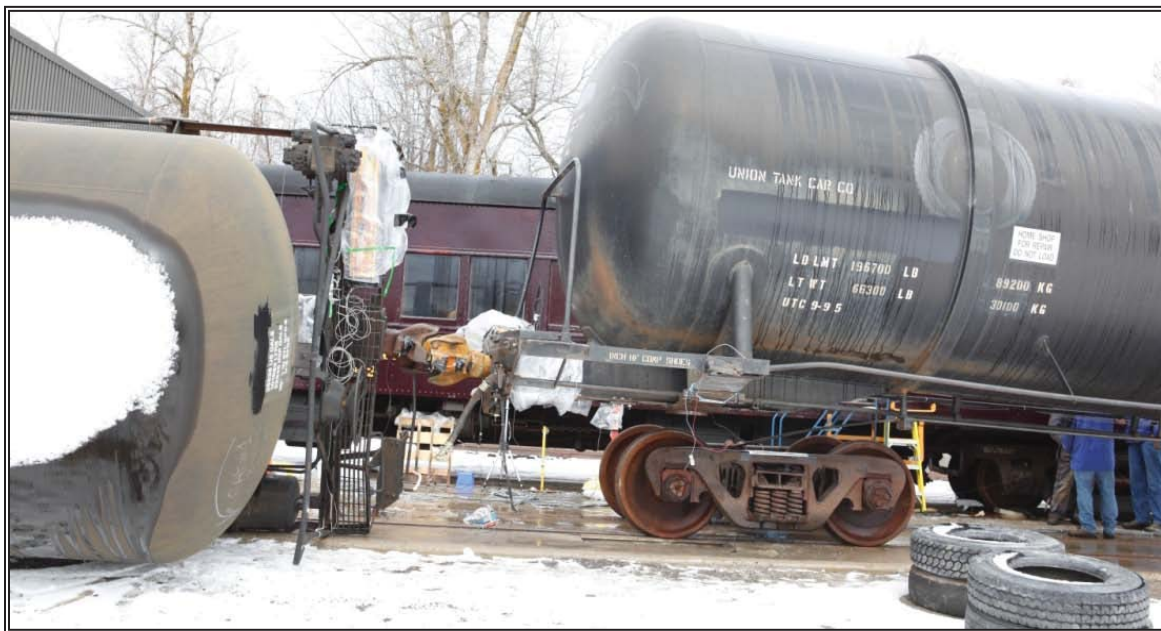
Figure 80: Test #2, cars after test, south side – modified rotary coupler junction.
