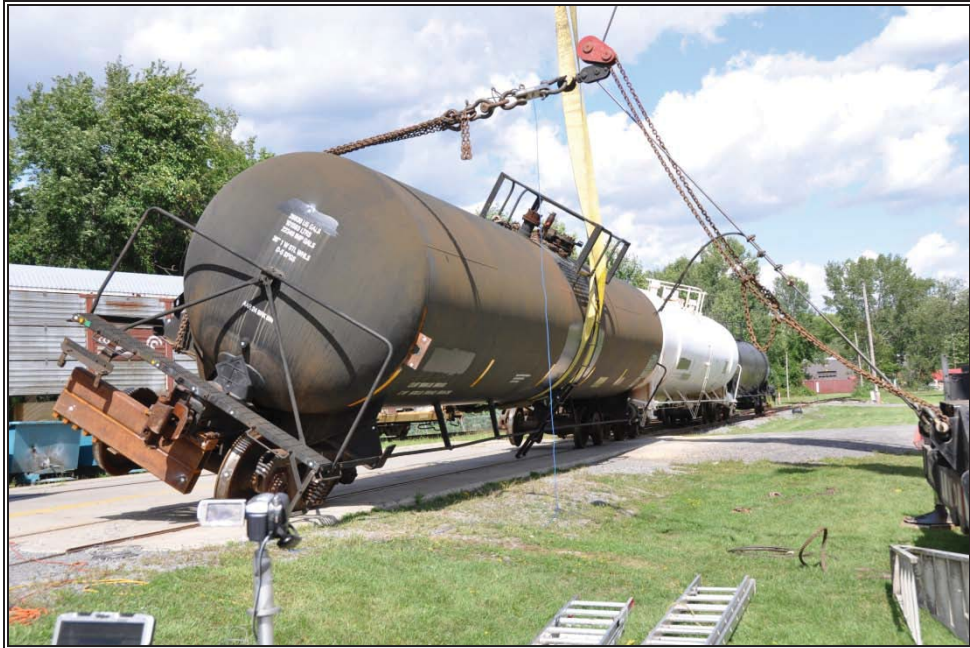
Figure 33: Pulling laterally at the end of the car from top.
