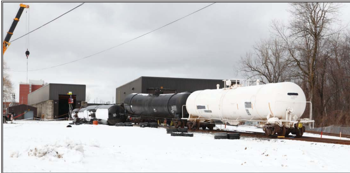
Figure 78: Test #2, cars after test, tail end – rotary coupler stopped the rollover propagation.
