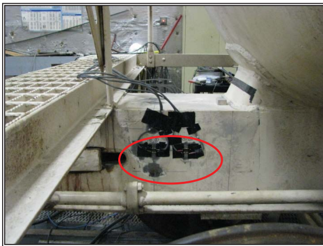
Figure 49: Typical strain gauge locations to measure car vertical load and torque.
