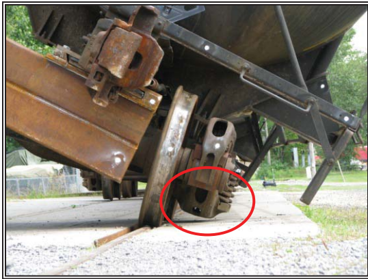
Figure 37: Truck almost touching the concrete during the dry-run test (left); and holes in the concrete during testing (right).
