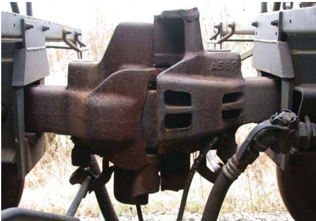
Figure 8: Double shelf couplers mated together showing height mismatch due to different coupler centreline heights, and a drooped coupler on the left car.
