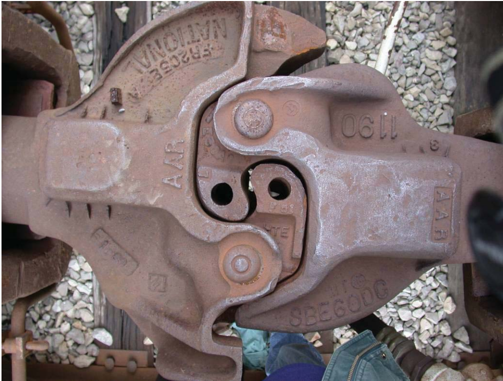
Figure 26: F-type rotary coupler (left) mated with non-rotary E-type coupler (right).
