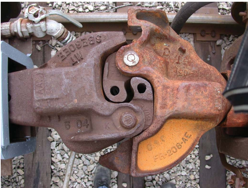
Figure 25: F-type rotary coupler (right) mated with non-rotary E-type coupler (left).
