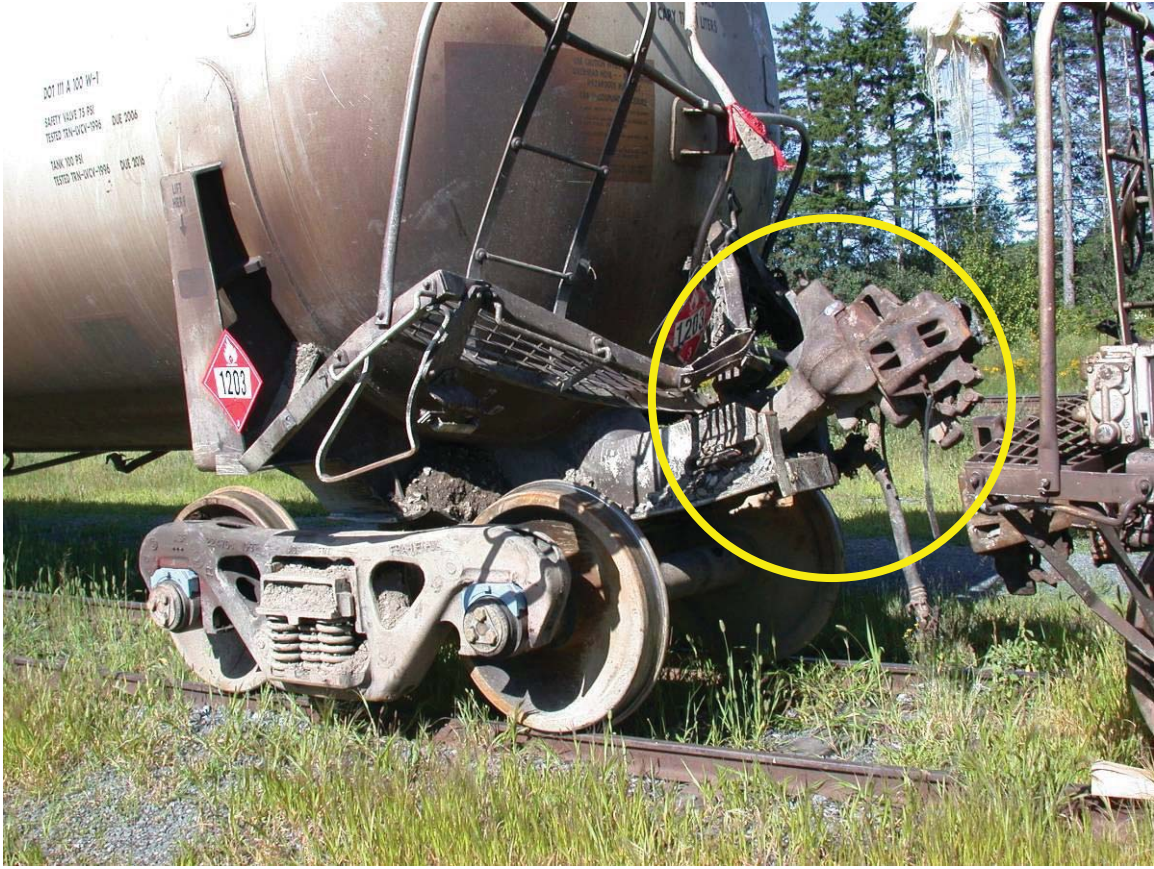
Figure 19: Coupler and end walkway bent up after derailment.
