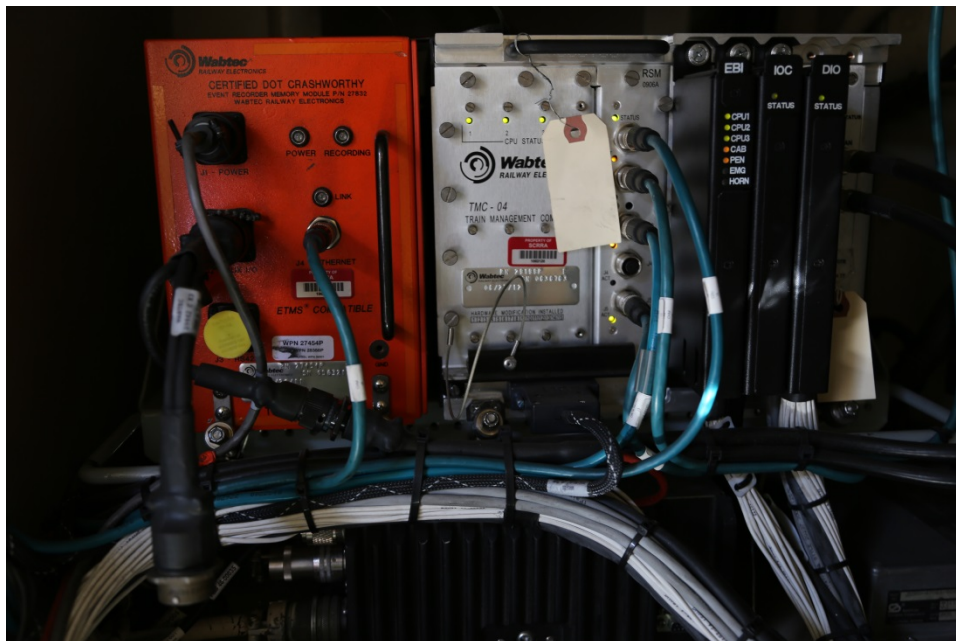
Figure 1. TMC and Event Recorder placement in Locomotive 870.
