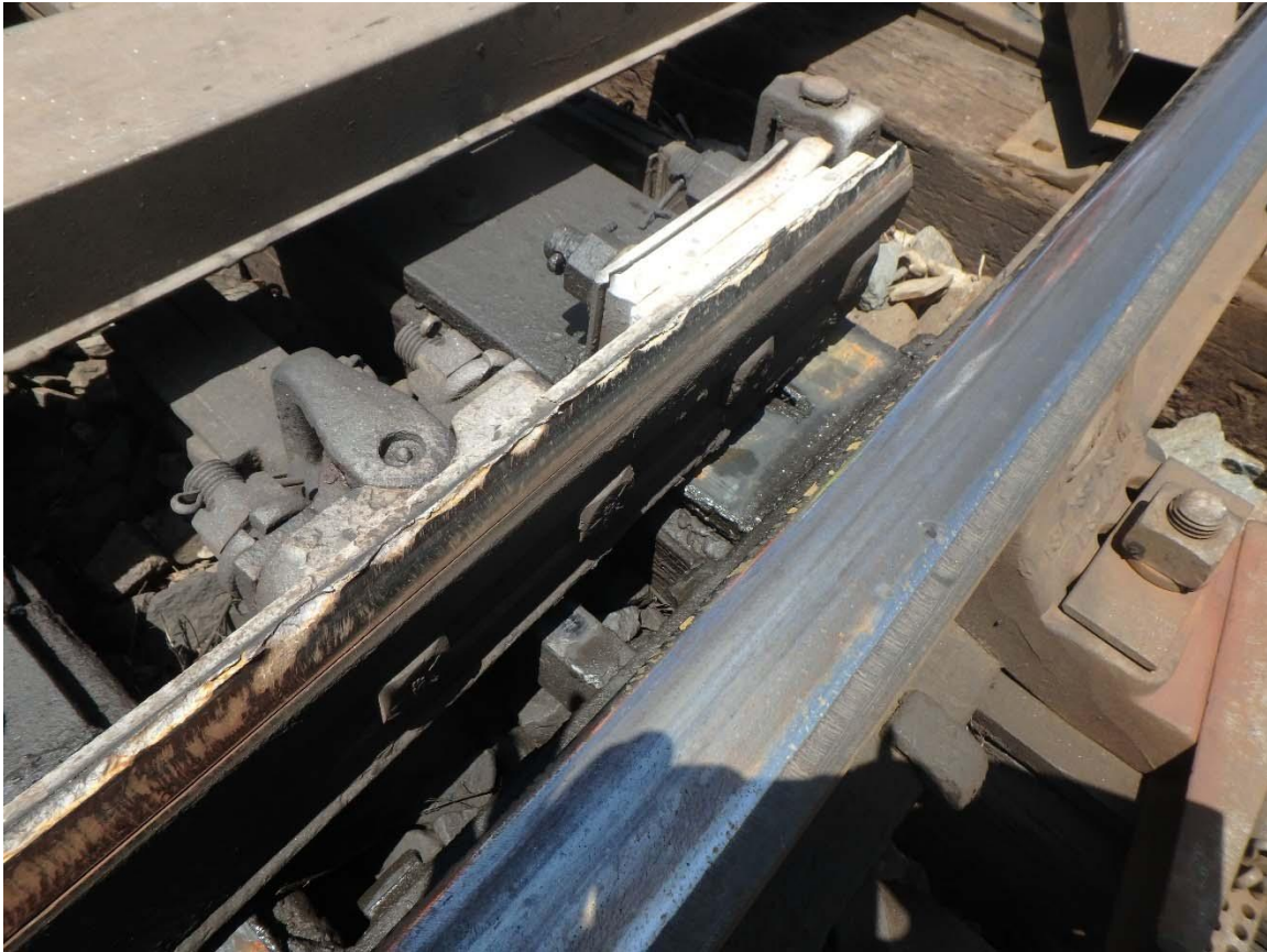
5 Figure 4. Metal flow chipped from back side of left hand switch point indicating a run through switch 6 condition. Photo shows railroad switch components. (Photo NTSB)
