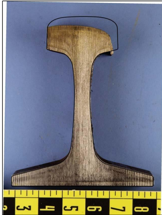
Figure 10. Photo of cross section of rail near 12N. Outline shows loss (wear) of rail hear.
