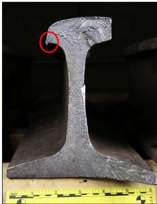
Figure 10. Photo of cross section of rail near 12N. Outline shows loss (wear) of rail hear.
