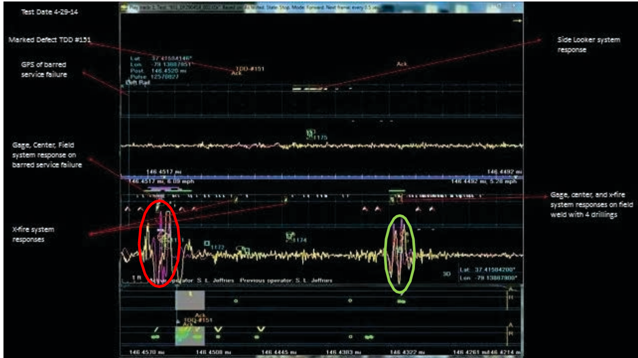
Figure 12. Screen image of the rail test data for MP 146.45.
