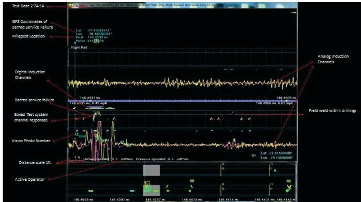
February rail test—10 foot screen shot, rail joint bar at MP 146.46, no rail defects.
