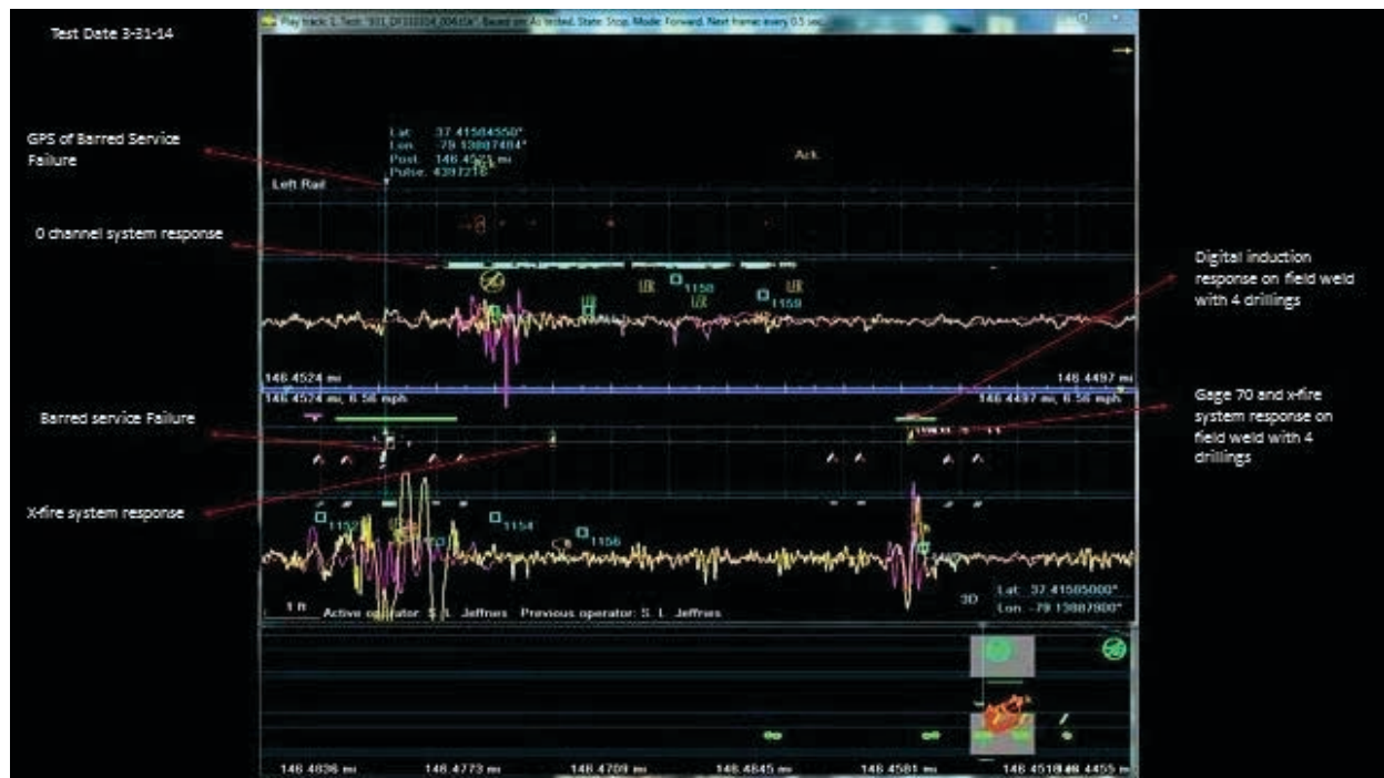
March rail test---10 foot screen shot, rail joint bar location at MP 146.45. No rail defects.
