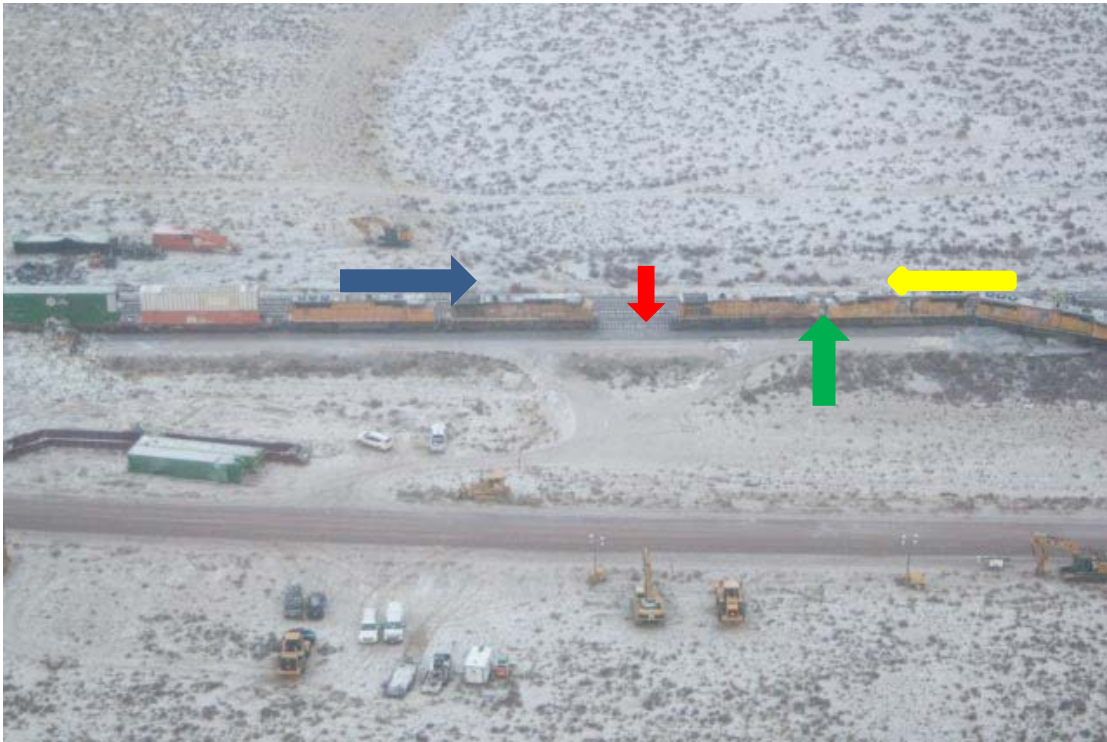
Figure 1. This is an aerial view on March 15, 2016, looking south at the derailment area. The red downward arrow identifies the point of collision (impact); the yellow arrow shows the position and EB direction of travel of the stopped local train, LCK41; the blue arrow identifies the WB direction of travel of the striking train; the green upward arrow identifies the “as found” position of the locomotives. Note: the striking train moved the stopped train about 246’ west.
