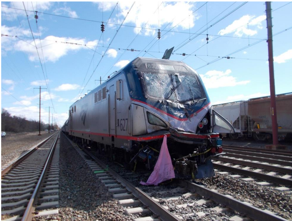
Figure 1. A view at the resting position Amtrak 627 on main track 3. Note the damage to the front of the locomotive, window damage can be seen on the west side of the first passenger coach.
