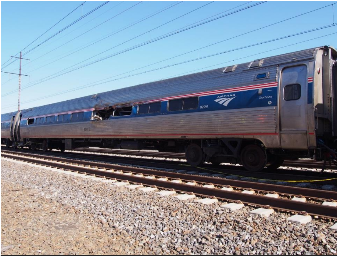
Figure 5. This is a view of the damages on the west side of the first passenger coach car.
