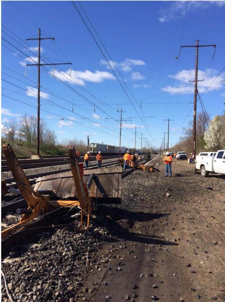
Figure 2. This is a view looking south at the scattered debris from the train strike of the MOW equipment.
